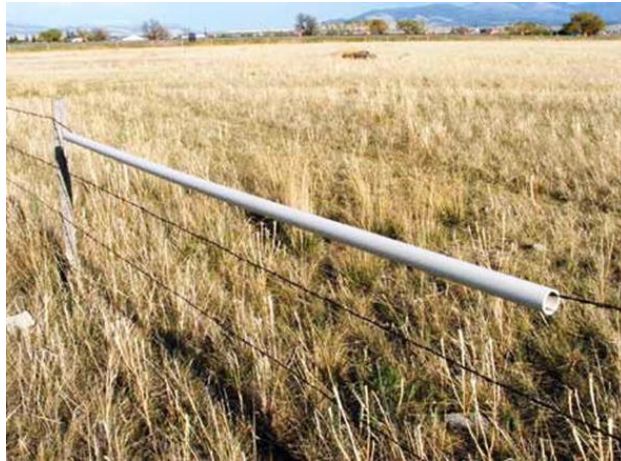
Figure 5. Top wire fence modifications: Wildlife friendly fence modifications deployed on the top wire of multi-stranded barbed wire fencing during second set of field trials. These included sage grouse markers (A.) and PVC pipe (B.). Top wire modifications were placed at known crossing during the after periods of field trials.
