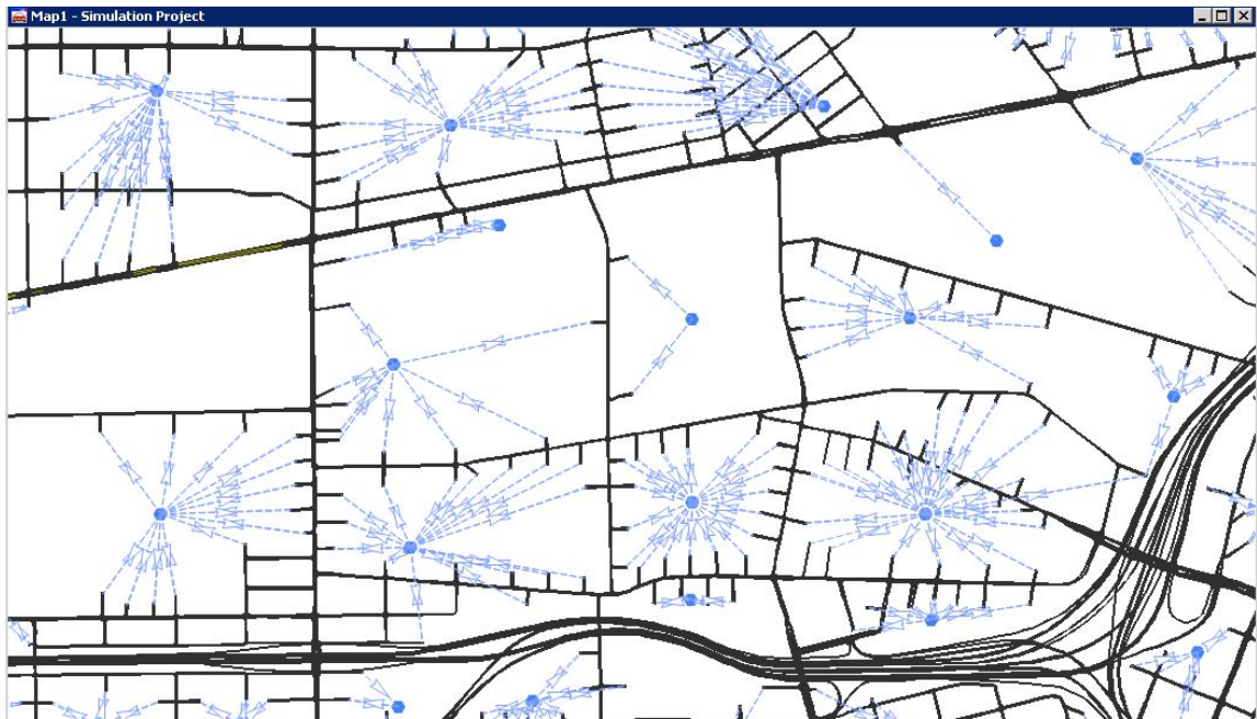
Figure 5. Connectors to approximate parcel loading.
