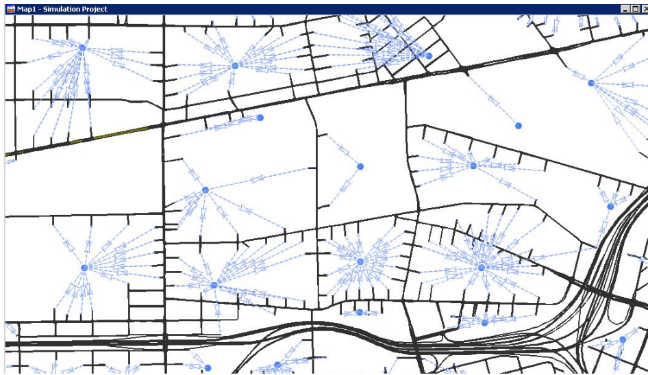
Figure 7. Connectors to approximate parcel loading.
