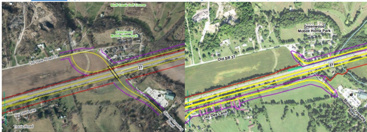
Figure 7: The Refined Preferred Alternative (right) includes a service road south of the highway that was not included in Alternative C4 (left), enhancing local accessibility and connectivity. (Images courtesy of Indiana Department of Transportation)
