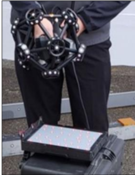
Figure 18. Photograph. Handheld scanning device used during the TPP equipment rodeo to establish ground reference data.
