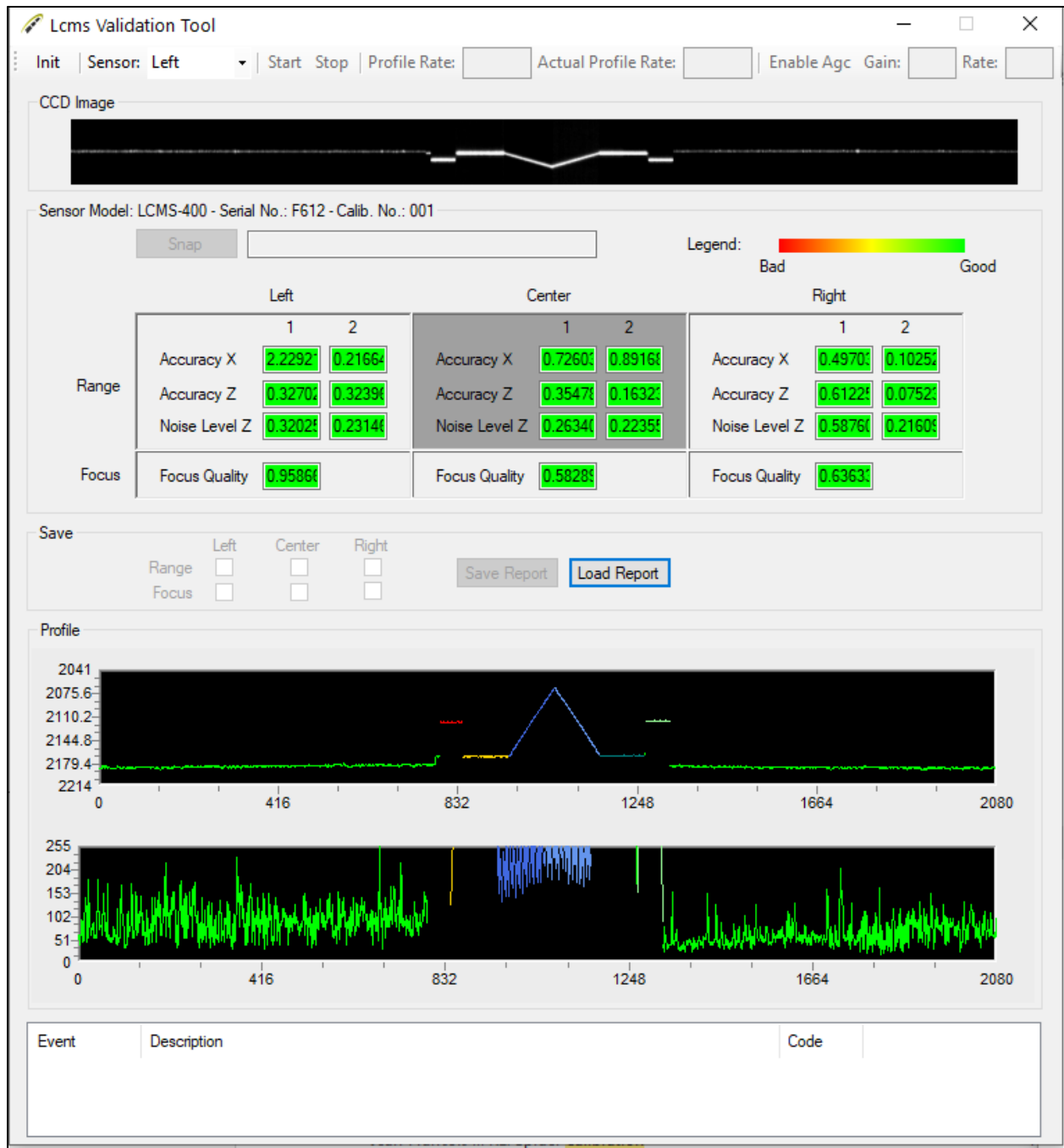
Figure 33. Illustration. Example of LCMS Validation Tool software being used to check data quality using the LCMS Validation Object.
