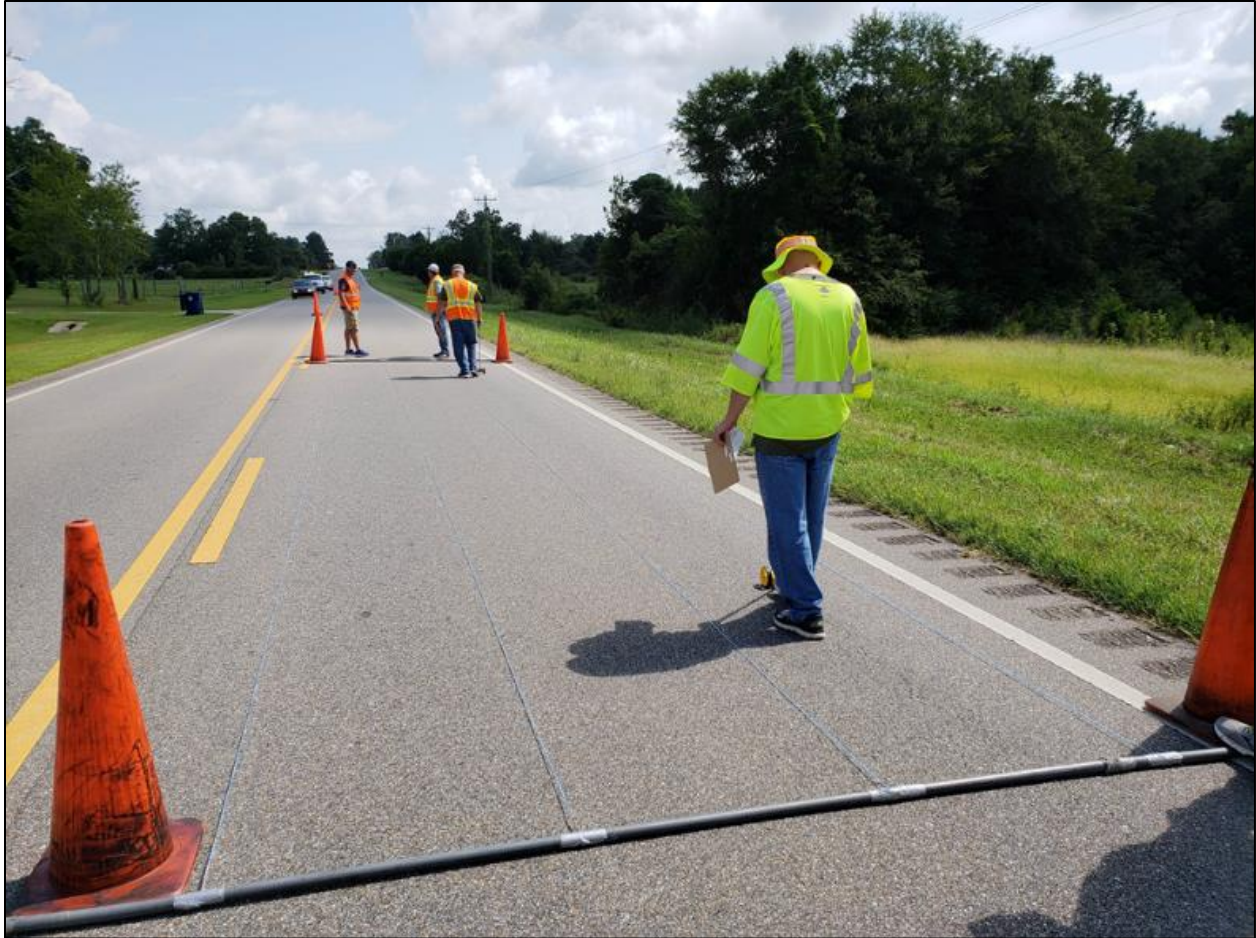
Figure 25. Photograph. A template that may be used to increase the efficiency of wheel path layout taken from the draft report developed under Developing TPF-5(299)/(399) Guidelines for Cracking Assessment for Use in Vendor Selection Process for Pavement Crack Data Collection/Analysis Systems and/or Services.
