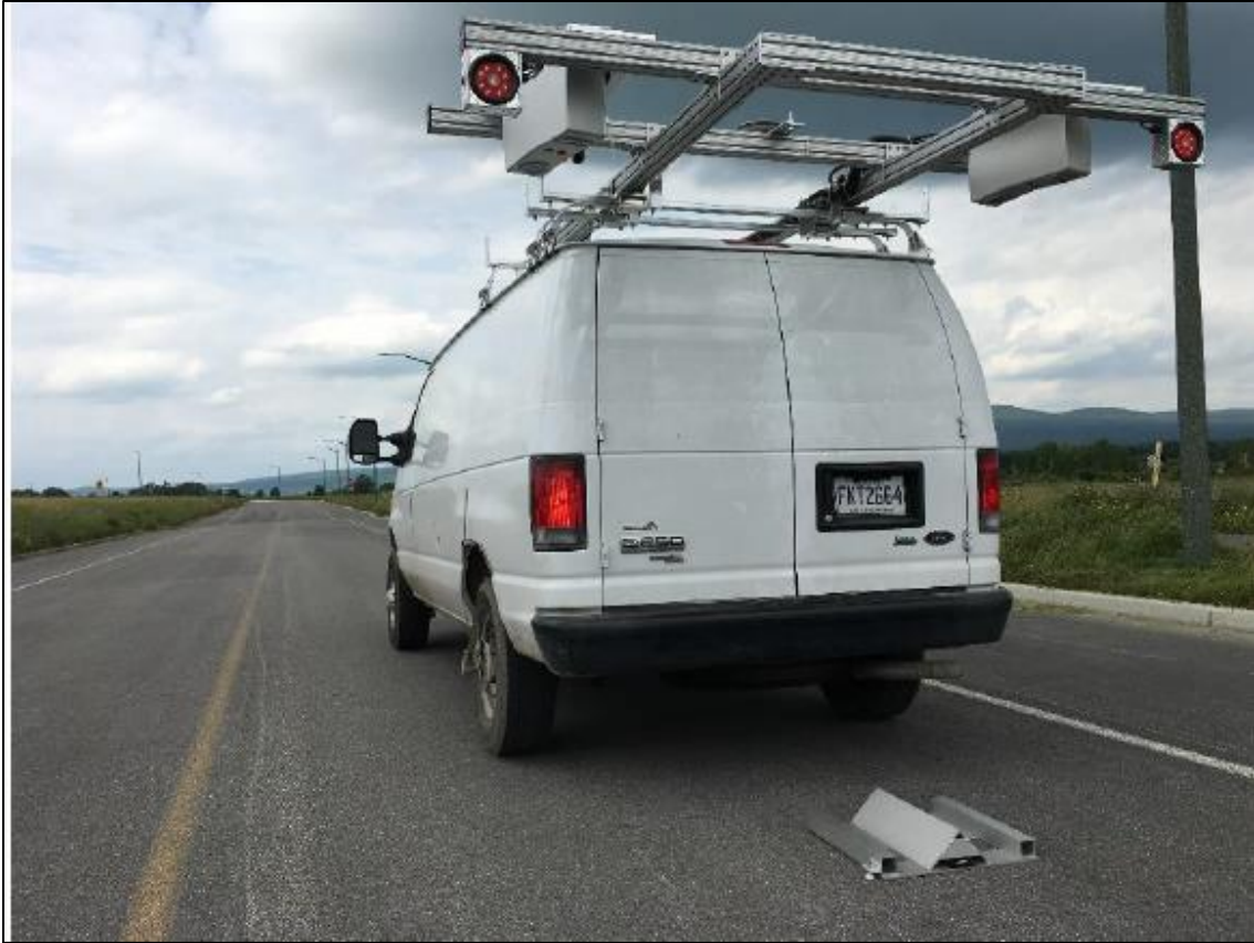
Figure 31. Photograph. Example of LCMS Scanning of the Validation Object.
