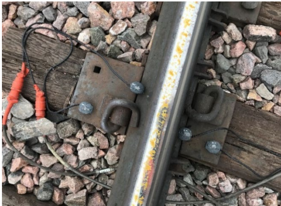
Figure 1. Instrumented spikes in a tie plate
