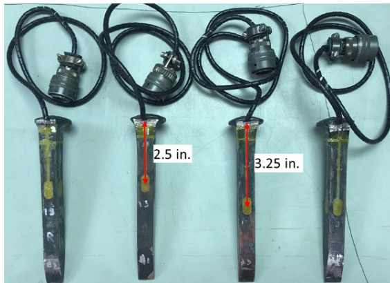
Figure 2. Instrumented locations of strain gages
