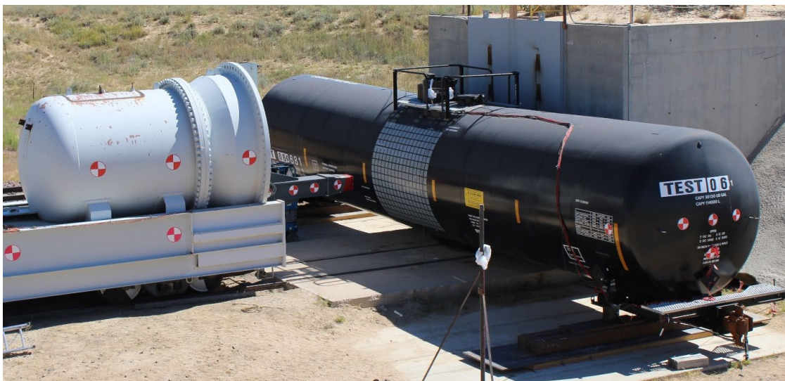
Figure 2. Shell Impact Test Setup (DOT-117 Shown)
