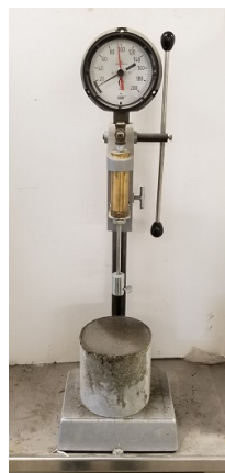
Figure 33. The loading apparatus for evaluating set time of concrete
