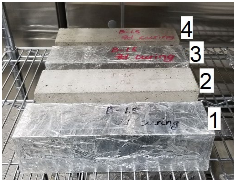
Figure 38. Free shrinkage specimens at four different conditions
