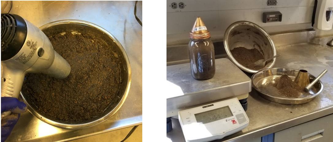
(a) Bringing aggregates to SSD condition (b) Cone mold for examining moisture condition of LWFA
