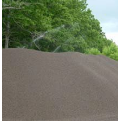
Figure 16. Sprinkler system used for soaking LWFA prior to batching
