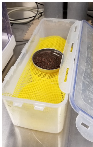
(b) Aggregates being tested for desorption
