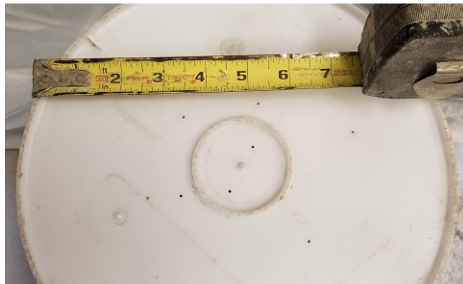
Figure 27. Openings at the bottom of the bucket for saturating LWFAs
