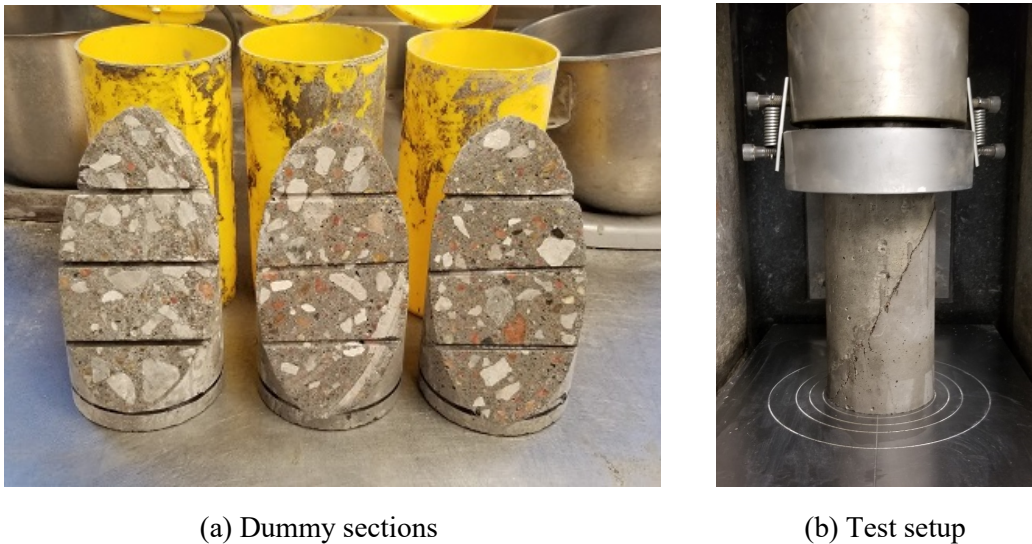
Figure 37. Bond strength test specimen and setup
