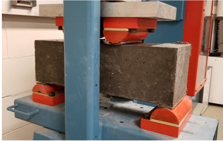
Figure 35. Test setup for flexural strength test
