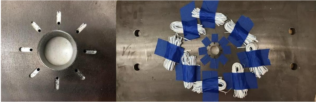
Figure 1. Drilled strain gage holes (left) and base plate with instrumented eight bolt strain gages (right)
