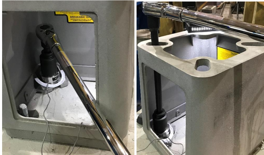
Figure 23. Tightening through the access hole (left) and tightening using the extension from the top (right)
