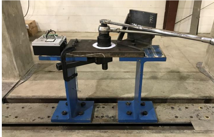
Figure 4. Anchor nut tightening performed on a 2 in anchor rod
