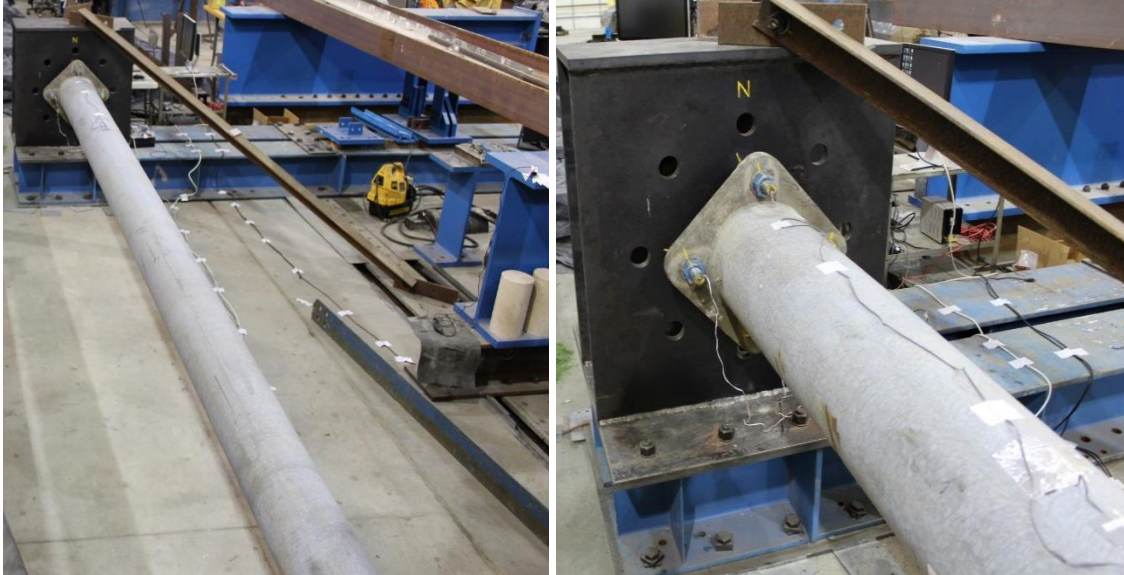
Figure 10. Complete view of the test-setup for large-scale testing
