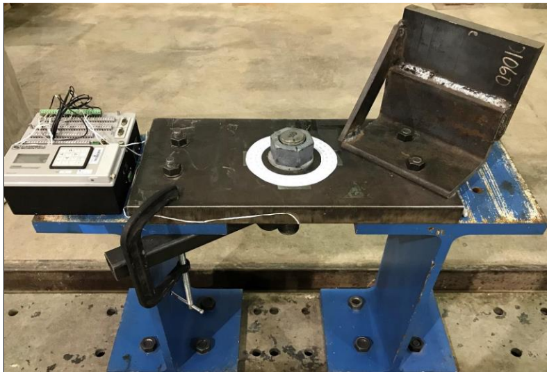
Figure 2. Test-setup for tightening anchor rods
