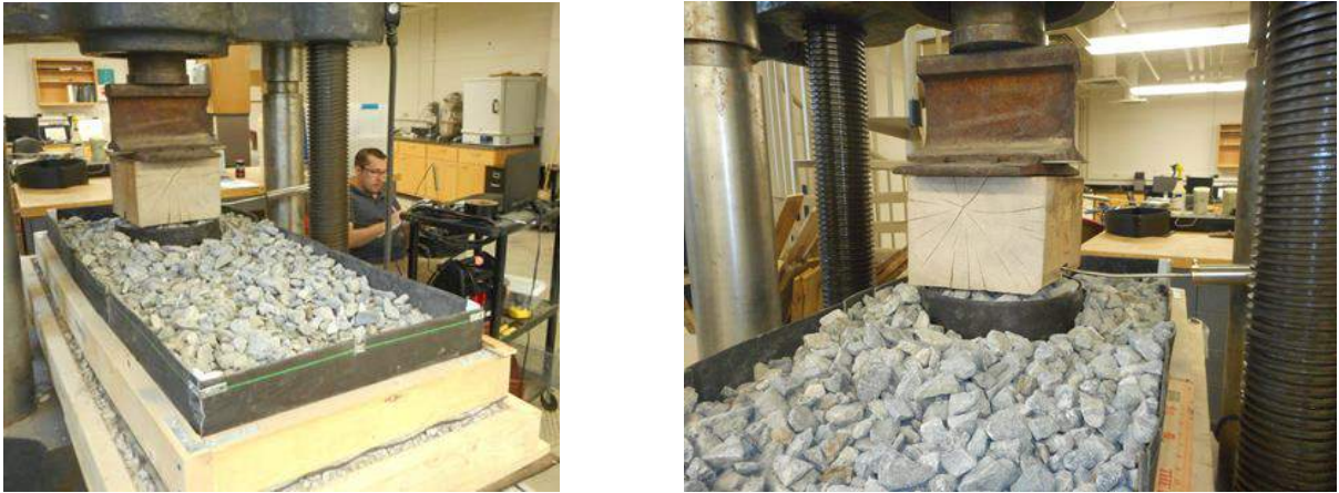
Figure 4. Track section and support used for laboratory tests.
