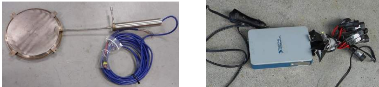
Figure 3.1.1. Pressure cell (left) and data logger module (right).
