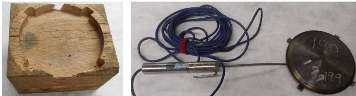
Figure 3. Routed tie section (left) and pressure cell (right).
