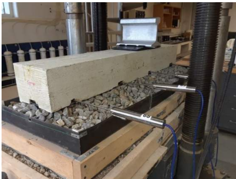
FIGURE 3.2. Half-Length Crosstie in Laboratory Setup (4)
