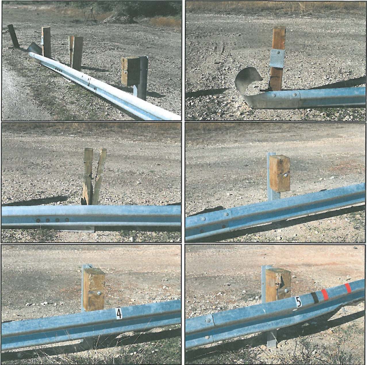
Figure 7.4. Posts 1 through 5 after Test No. 608331-01-6.
