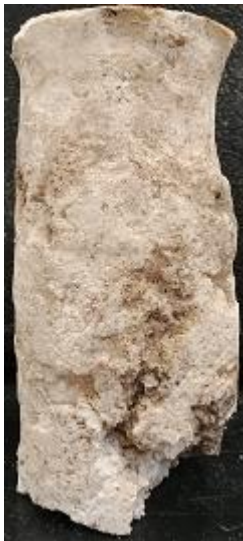
Figure D-3. Specimens deformed at 3,000 psi chamber pressure
