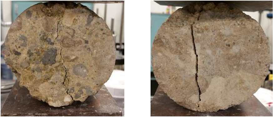
Figure 3-5. Examples of center splitting
