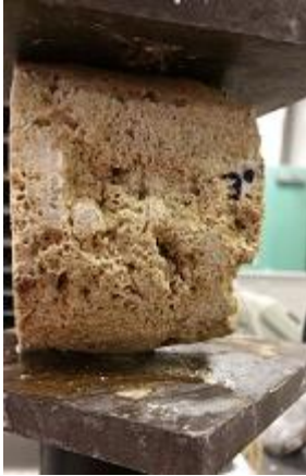
Figure 3-10. q_t test on sample 624-3 with uneven diameter
