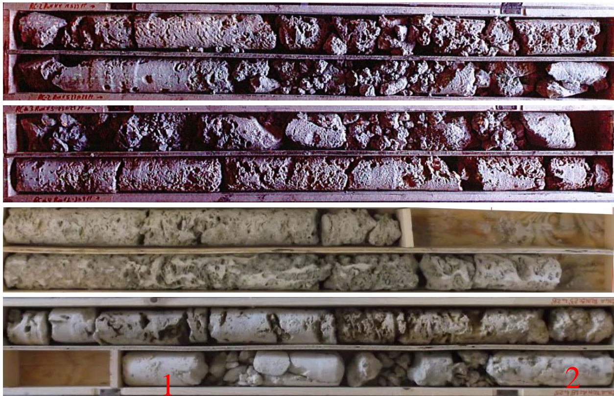
Figure 2-6. Examples of core runs with low RQD
