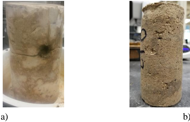
Figure 6-18. Outlier extension test specimens: (a) Hole on specimen; (b) One end of specimen is much softer
