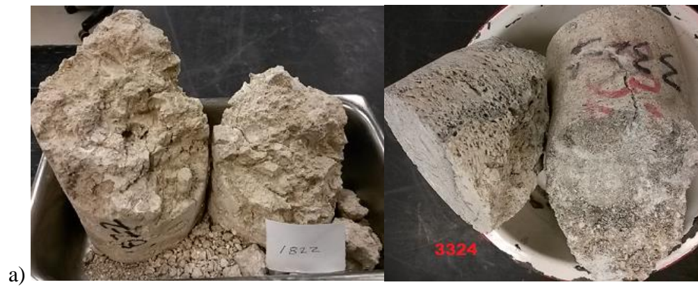
Figure D-2. Specimens tested at 130-psi chamber pressure: (a) \gamma_{dt} > 130 pcf
