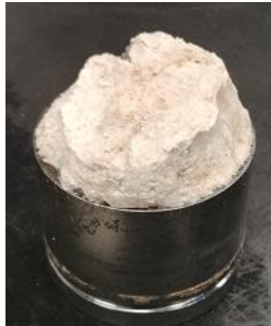
Figure D-3. Specimens deformed at 3,000 psi chamber pressure
