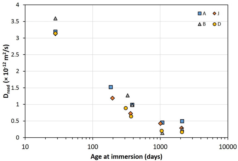
Figure 53. D_{nssd} vs. age at immersion measured on A, B, J, and D specimens
