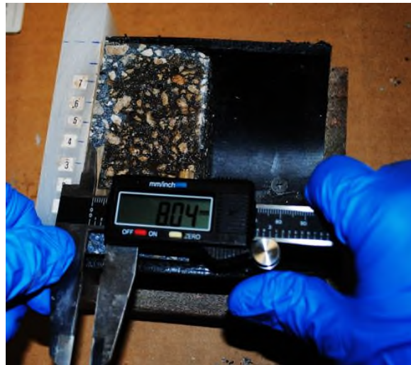
Figure 5. Measurement of chloride ion penetration depth.
