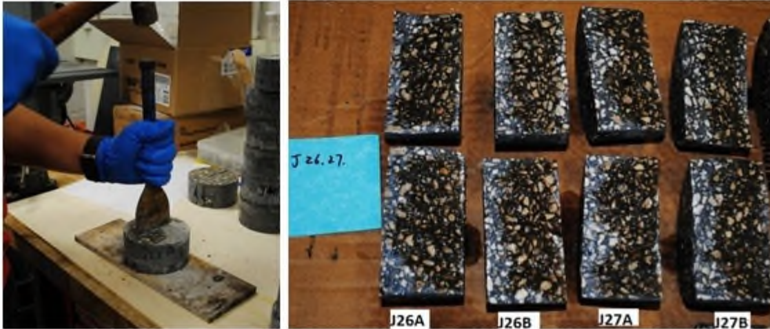
Figure 4. Illustration of splitting slices and spraying 0.1N AgNO 3 at the cross-section as an indication of chloride ion penetration depth.
