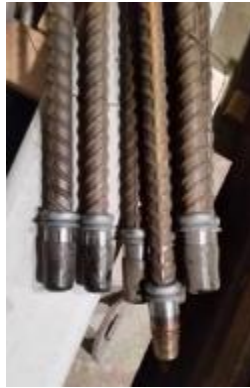
Figure 4.13. Threaded end of inclined reinforcement
