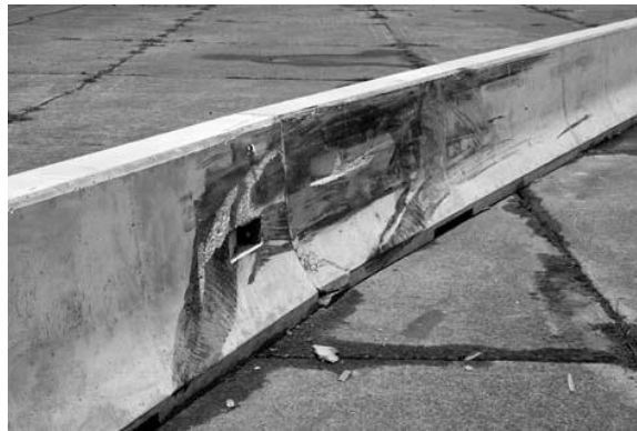
Figure 2.13. Damage to 30-ft long precast barrier with X-bolt connections
