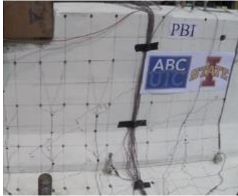
Figure 5.5. Test 1 (PBI middle) barrier cracks
