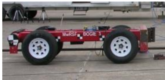
Figure 2.14. Impact bogie vehicle
