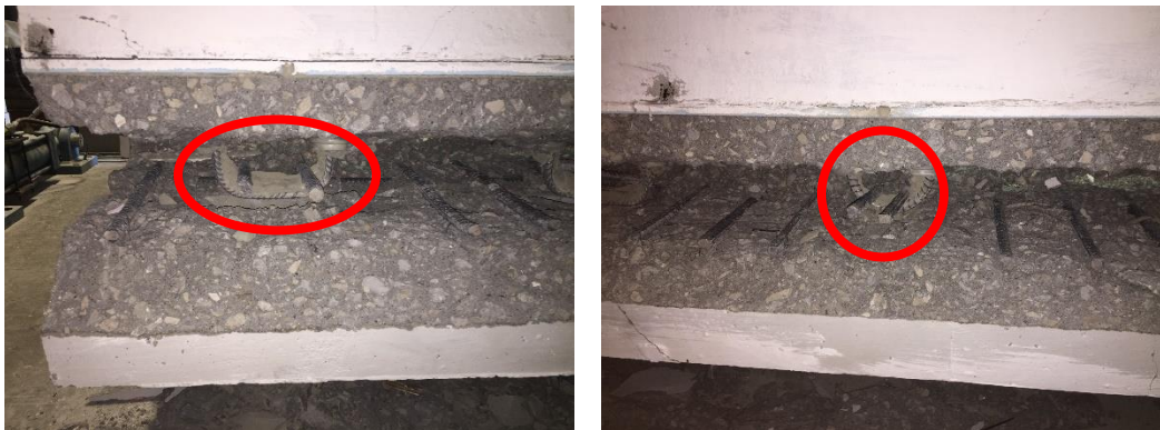
Figure 5.41. Top mat of the bridge deck reinforcement after the Test 6 pull test
