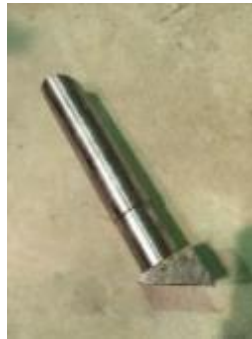
Figure 4.6. Inclined bar connection in deck
