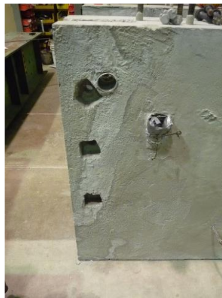
Figure 4.16. Pockets used to install transverse barrier-to-barrier connection
