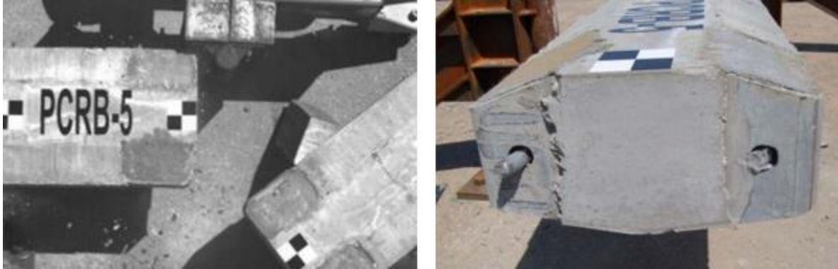
Figure 2.23. Alternate redesign I-shaped rail connection failure
