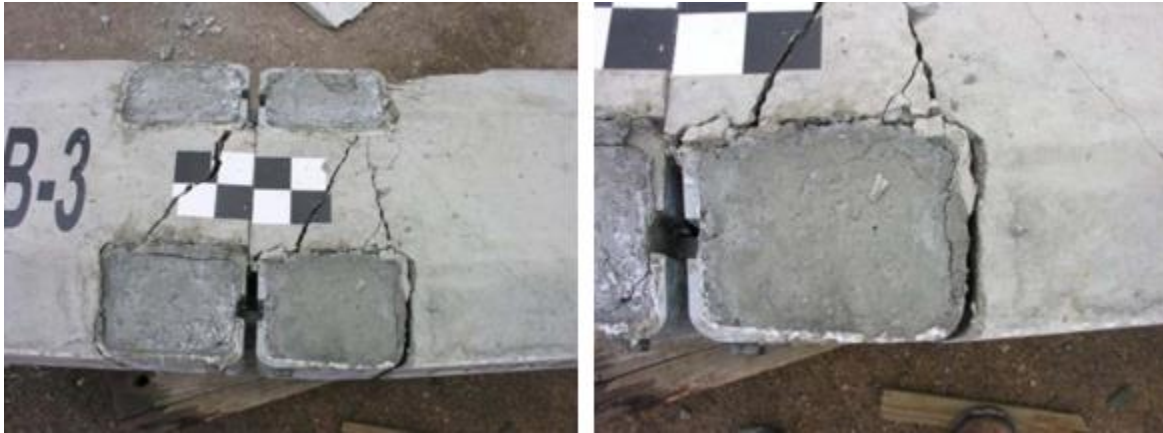
Figure 2.21. Redesign I-shaped rail connection after bogie testing
