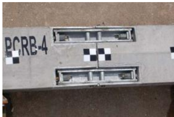
Figure 2.24. Side bolts and shear tube connection improvements
