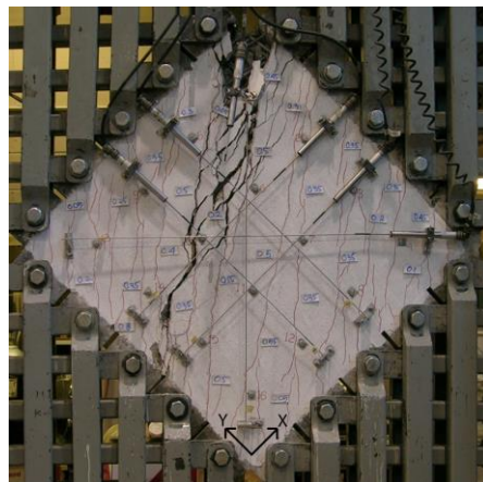
Figure 3.12 Failure crack pattern of RC panel C1C-R, (Susetyo, 2009)
