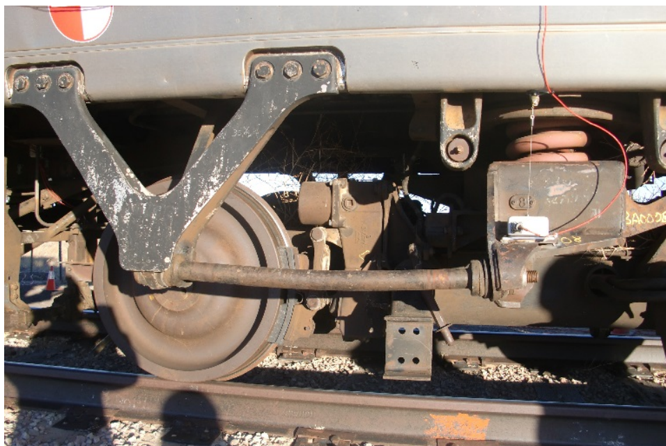
Figure 42. Bent Front Left Traction Bar
