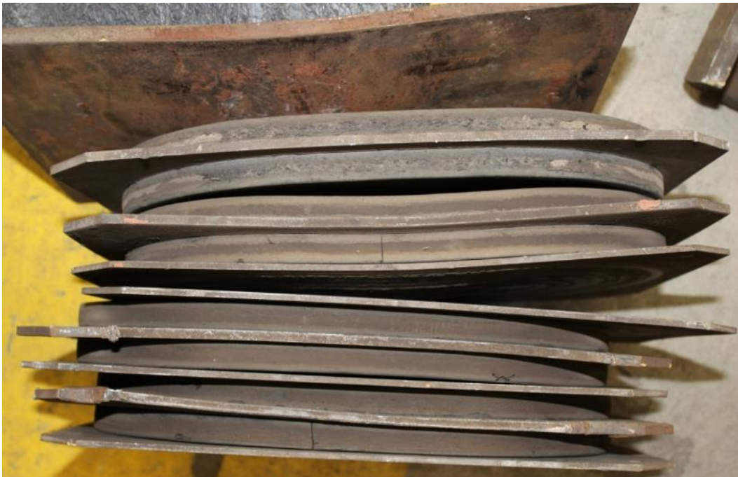
Figure 34. Bent Draft Plates
