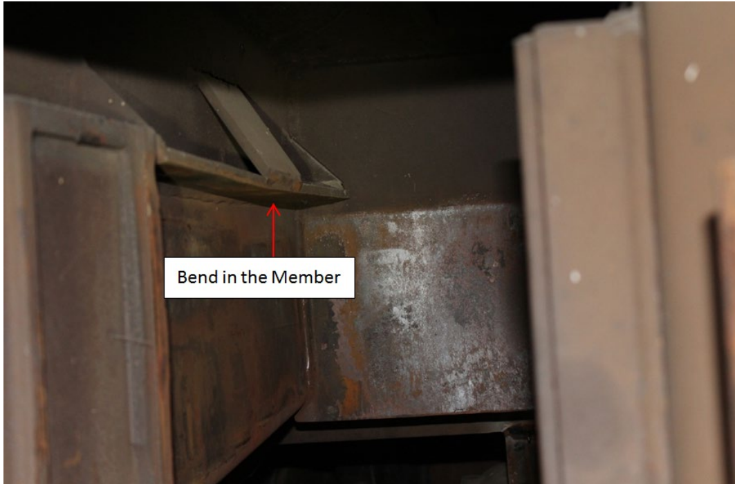
Figure 35. Bent Draft Pocket Member (right)
