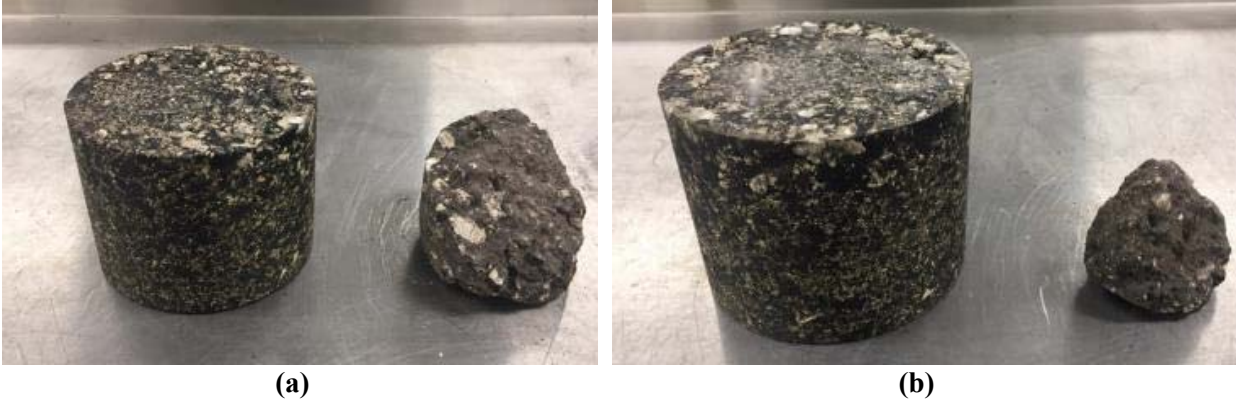
Figure 105. Specimens before and after Cantabro Abrasion Loss Test: (a) Mixture C-80L-LF and (b) Mixture C-60L-GF
