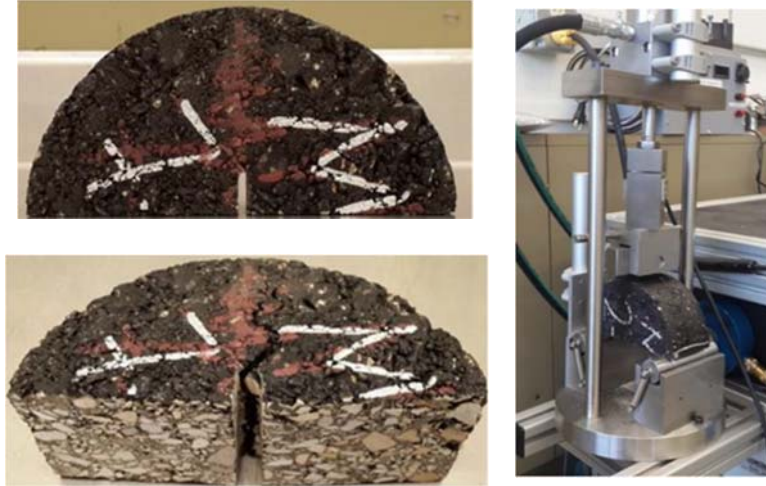
Figure 31. Semicircular Bending Test: (a) Notched Specimen before Failure, (b) Notched Specimen after Failure, and (c) Test Setup
