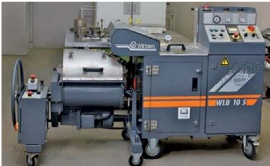
Figure 95. Wirtgen WLB 10S Foaming Unit
