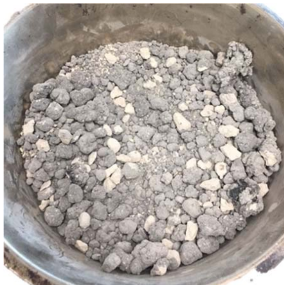
Figure 92. Appearance of Foamed Cold Recycled Mixture with 3% Foamed Binder and No MC after Mixing
