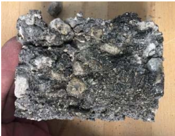
Figure 94. Cross-section of Foamed Cold Recycled Mixture Trial Specimen with 4% Foamed Binder Content and 4% MC
