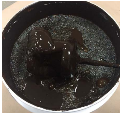
Figure K.4. Emulsion Sediment in Good Condition
