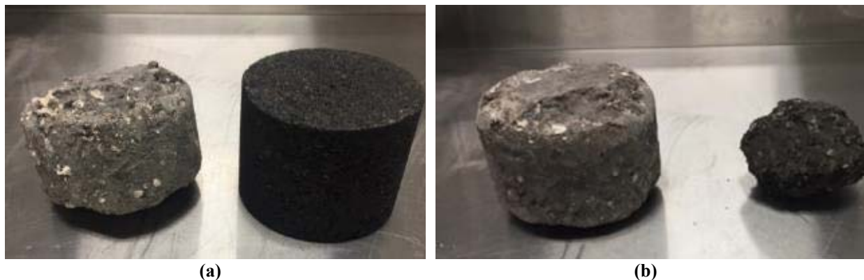
Figure 85. Cantabro Abrasion Loss Specimens: (a) Mixture C-60L-LE before (right) and after (left) Testing, and (b) Mixture C-60L-LE after Testing (left) and Mixture C-60G-GE after Testing (right)
