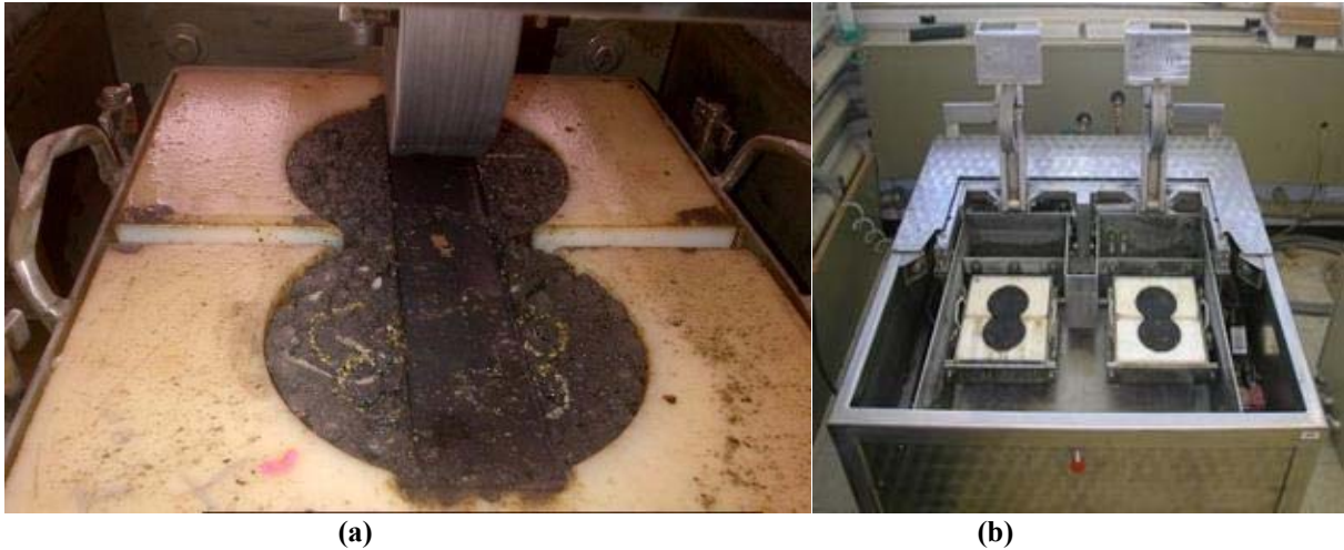
Figure 34. HWTT: (a) View of Loaded Specimens, (b) View of Apparatus
