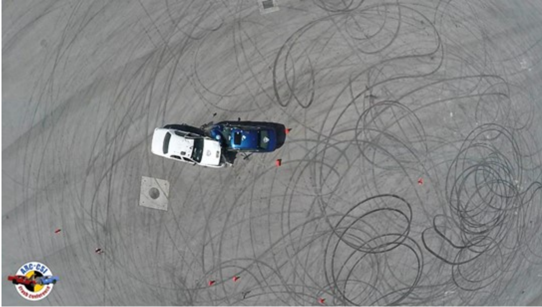
Figure 3.7 Overhead view showing the orientation of the test vehicles at impact.
