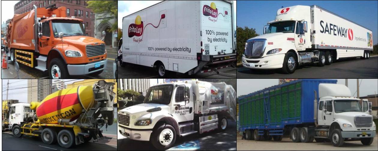
Truck LPDs are shown installed on single-unit as well as combination trucks. At top right, a rigid aerodynamic side skirt installed on a trailer. (Top right: Courtesy of Laydon Composites Ltd. All others: Alexander Epstein/Volpe, 2012-2015.)
