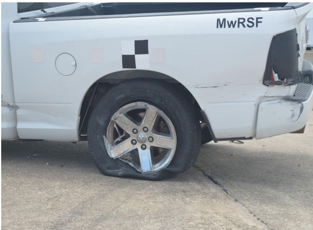
Figure 81. Left-Side Vehicle Damage, Test No. GSH-2
