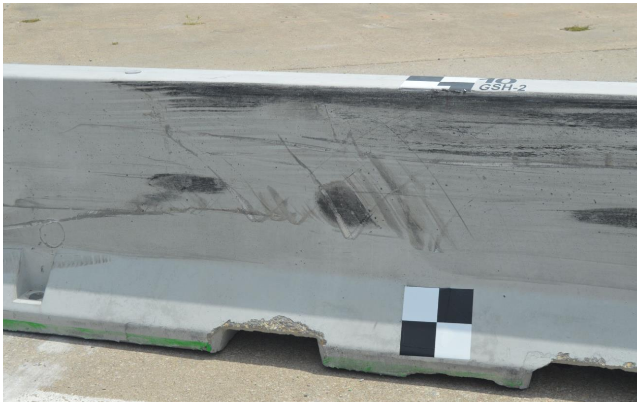
Figure 77. Barrier No. 10 Damage, Test No. GSH-2
