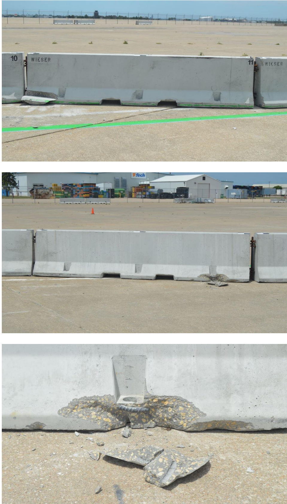
Figure 78. Barrier No. 11 Damage, Test No. GSH-2
