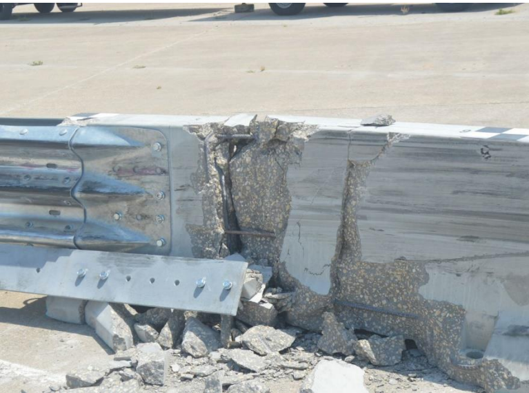
Figure 39. Barrier No. 9 Damage, Test No. GSH-1
