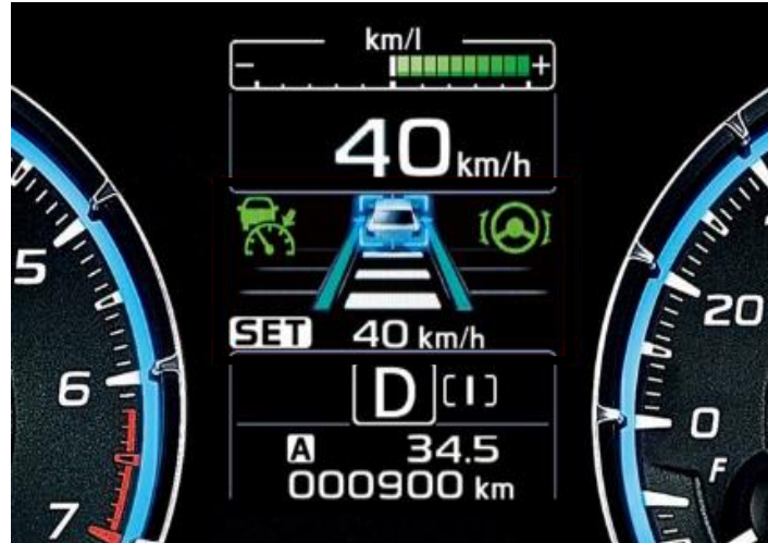
Figure 2-3. 2018 Subaru Levorg instrument cluster indicators.
