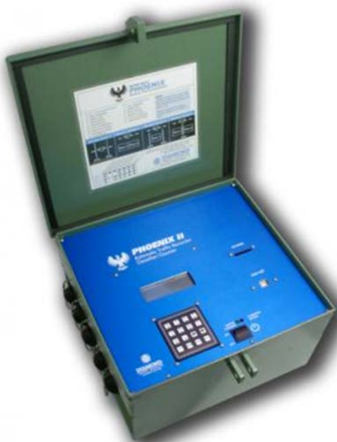
Figure 3-22 Phoenix II Diamond Traffic Unit.
