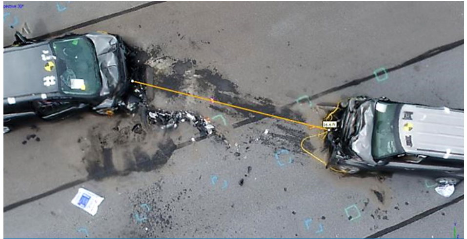
Using measurements from photos captured by unmanned aerial systems accelerates crash investigations.
