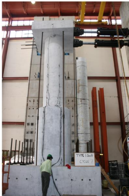
Fig. 2-10: Tests on column-oversized drilled shaft assemblies.
