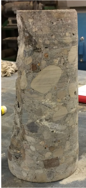
Figure 13 Sample from Pendleton County shown inhomogeneous and very poor gradation
