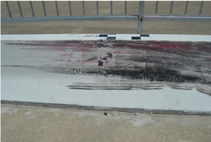
Figure 52. Tire Marks and Concrete Scraping, Test No. MNPD-3
