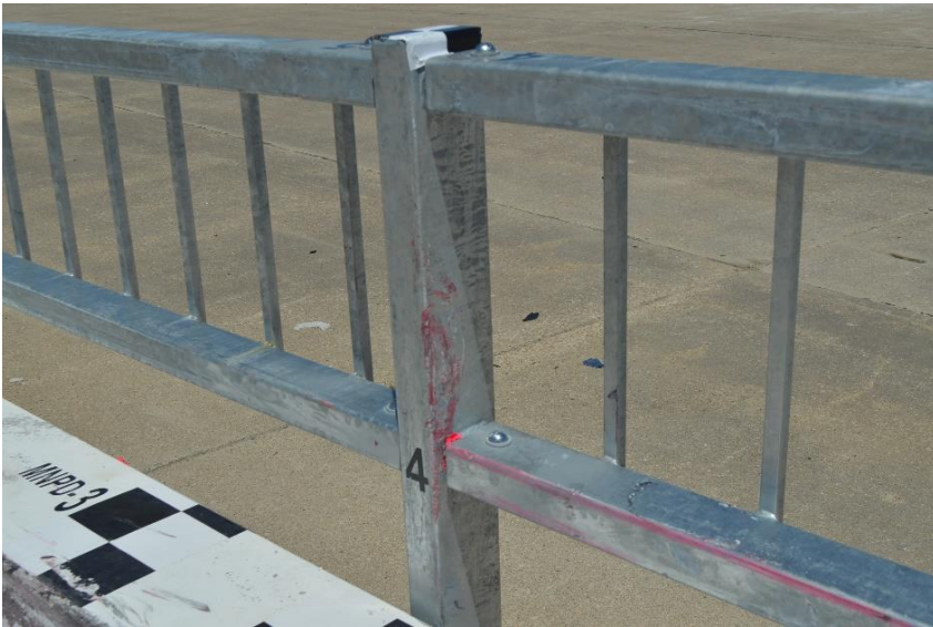
Figure 53. Rail and Post No. 4 Damage, Test No. MNPD-3
