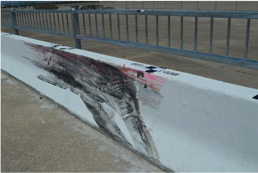
Figure 50. System Damage, Test No. MNPD-3
