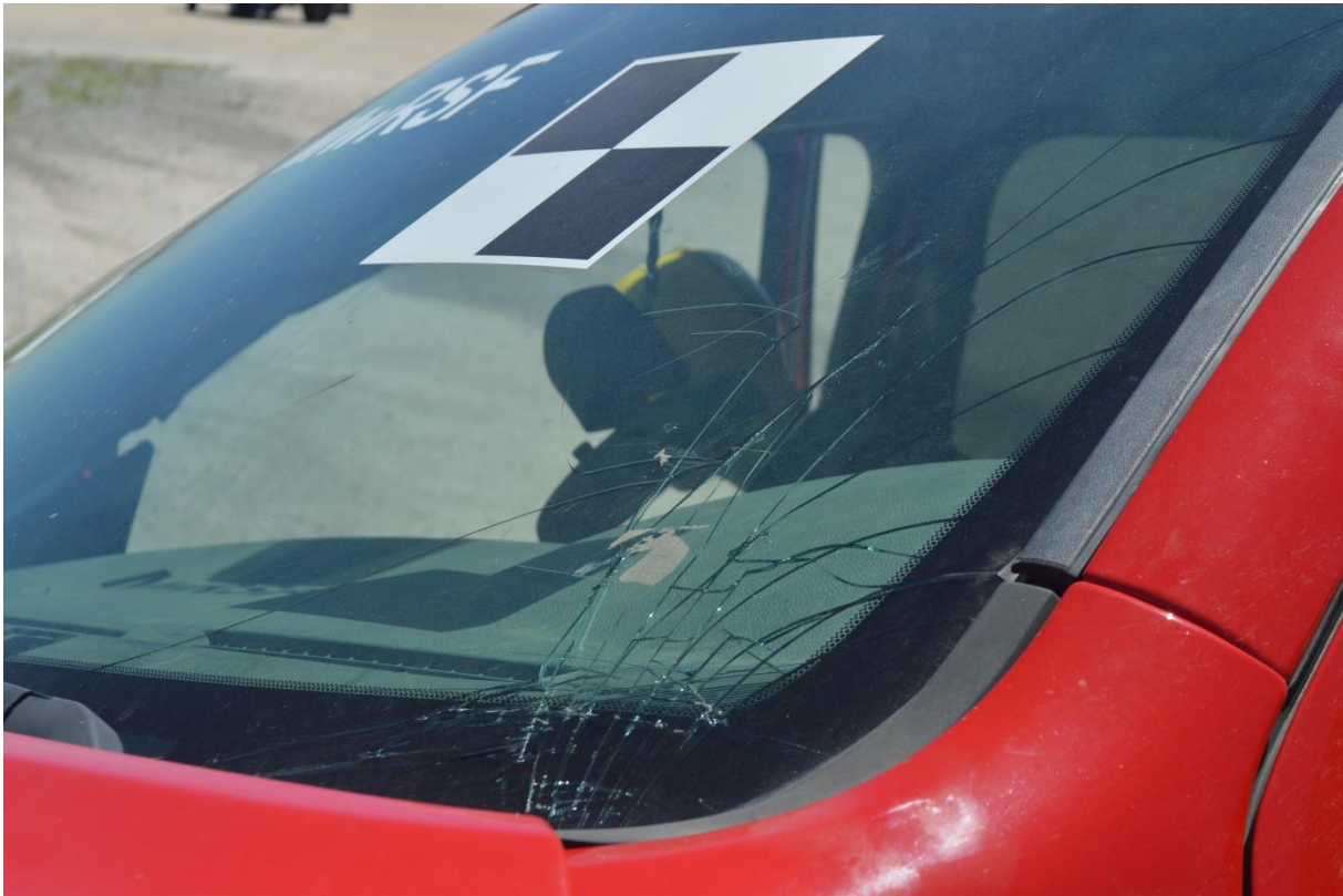
Figure 67. Windshield Damage (Post-Test), Test No. MNPD-3
