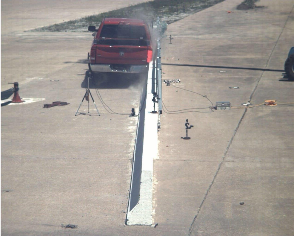
Figure 72. Downstream View of Head Ejection, Test No. MNPD-3
