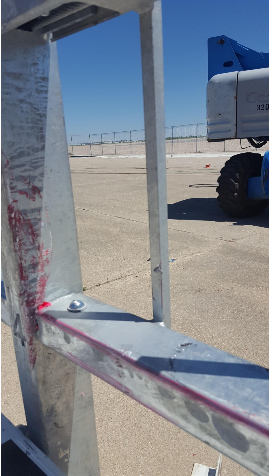
Figure 55. Spindle Contact and Debris, Test No. MNPD-3
