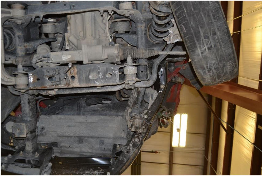
Figure 65. Undercarriage Damage, Test No. MNPD-3
