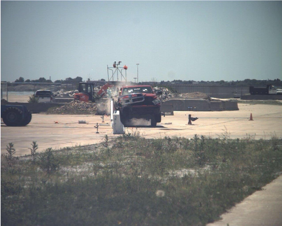
Figure 71. Upstream View of Head Ejection, Test No. MNPD-3
