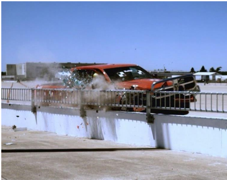
Figure 73. Angled Downstream View of Head Ejection, Test No. MNPD-3
