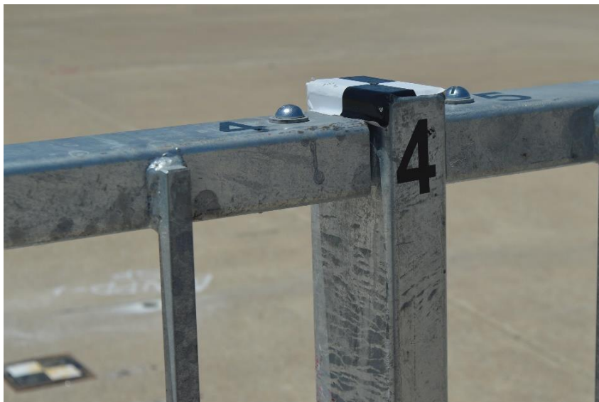
Figure 58. Rail and Post No. 4 Damage, Test No. MNPD-3
