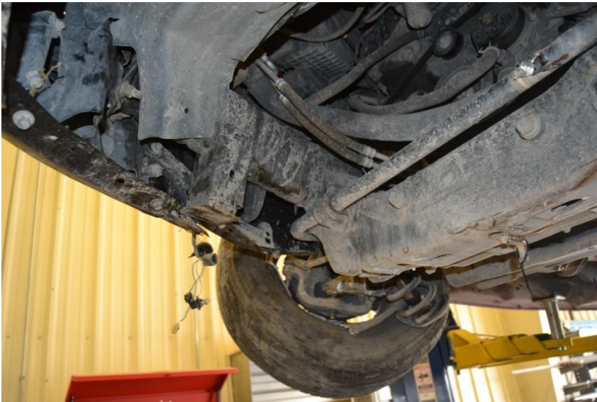
Figure 66. Undercarriage Damage, Test No. MNPD-3
