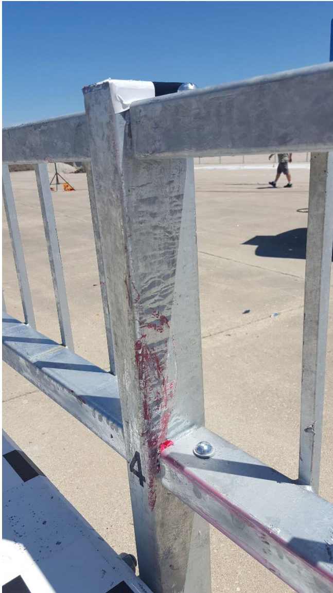
Figure 54. Rail and Post No. 4 Damage, Test No. MNPD-3
