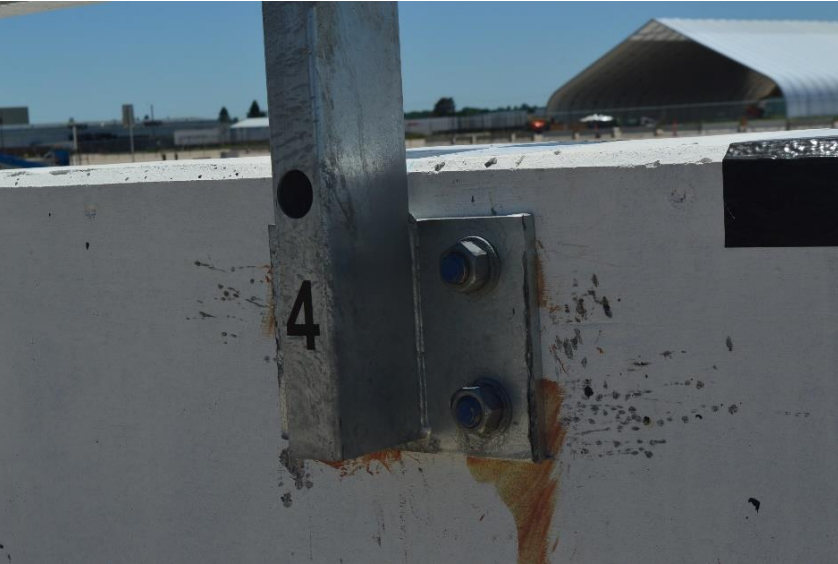
Figure 57. Rail and Post No. 4 Damage, Test No. MNPD-3
