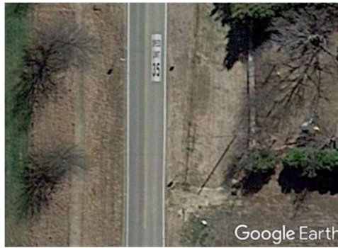
Speed limit pavement marking sign (Chitturi et al., 2017).
