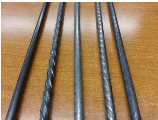
Figure 2: Five different 5.32-mm-diameter wires with different indentation types were utilized
