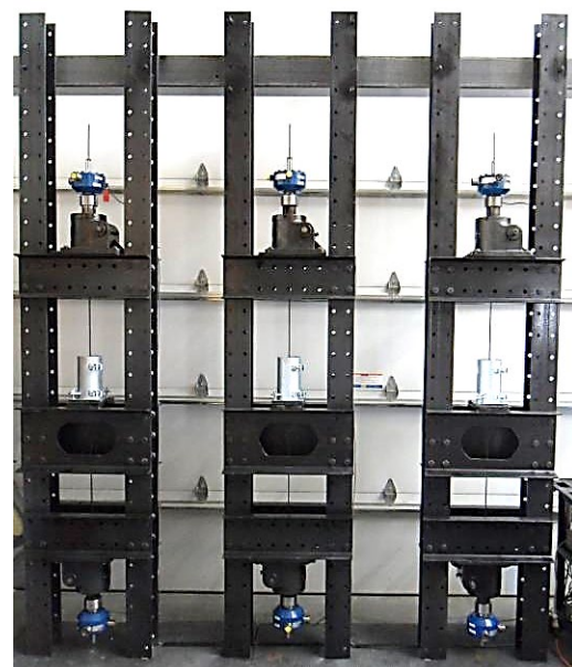
Figure 4: Three vertical prestressing frames
