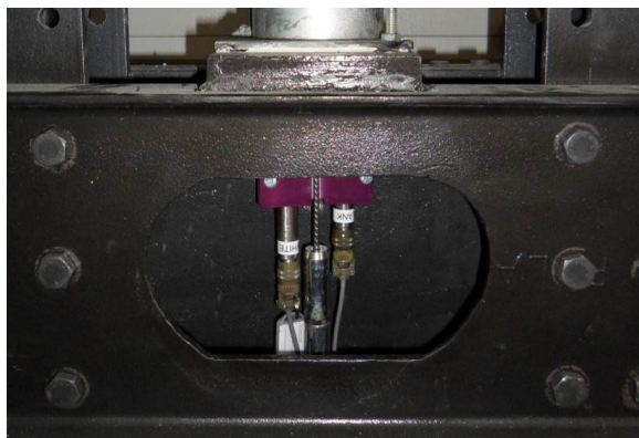
Figure 7: Two LVDTs measure wire slip with respect to the steel bottom plate of the concrete mold
