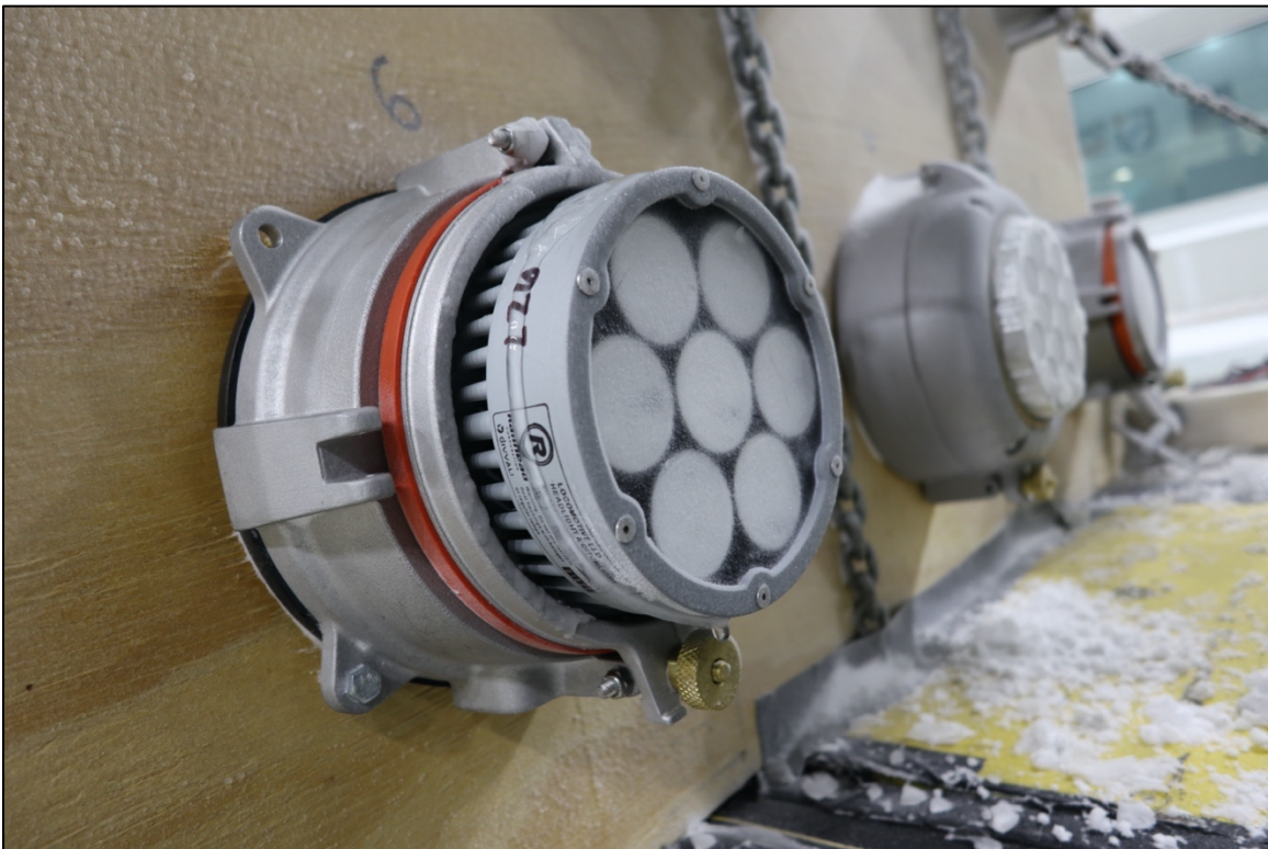
Figure 46. LED sample after Trial 2 (non-powered sample)
