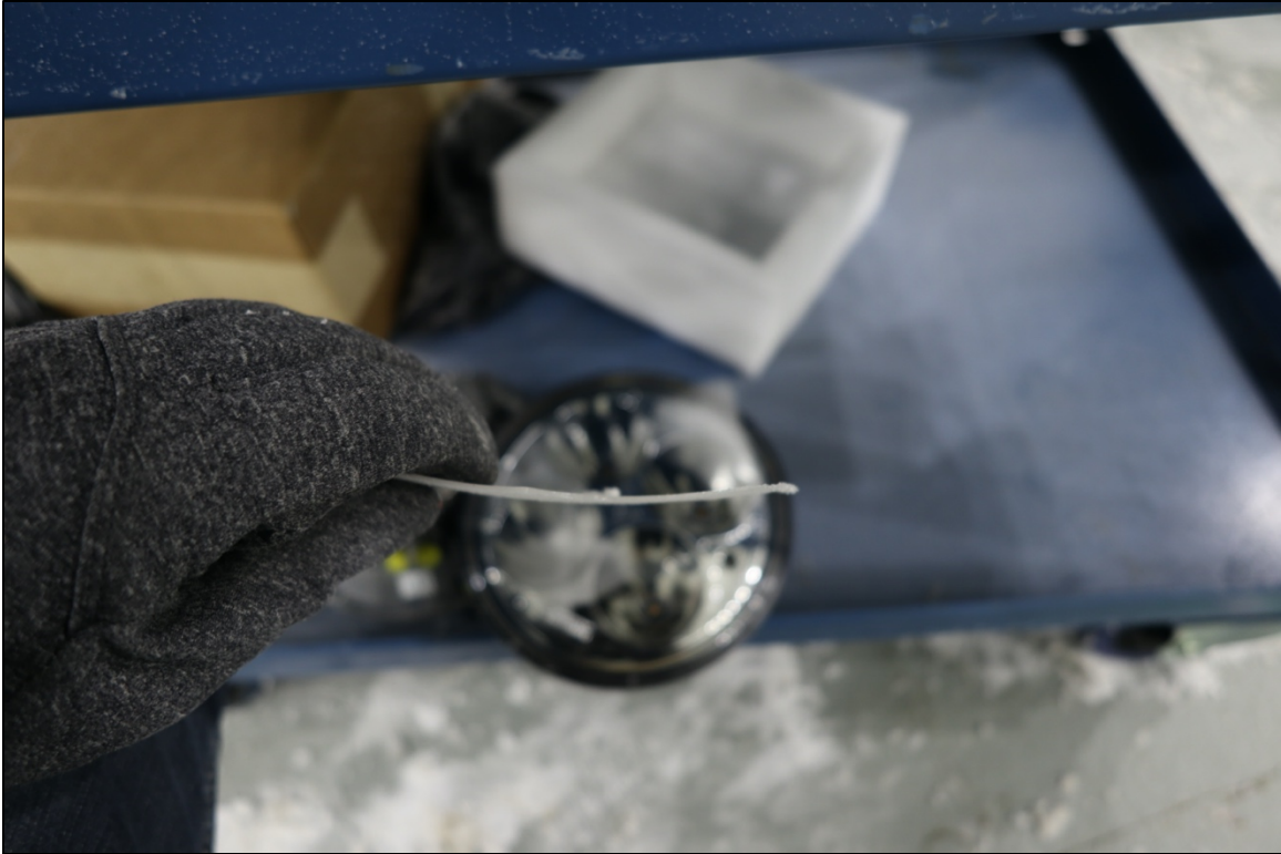
Figure 39. Measurement of ice accumulation on LED sample after Trial 1
