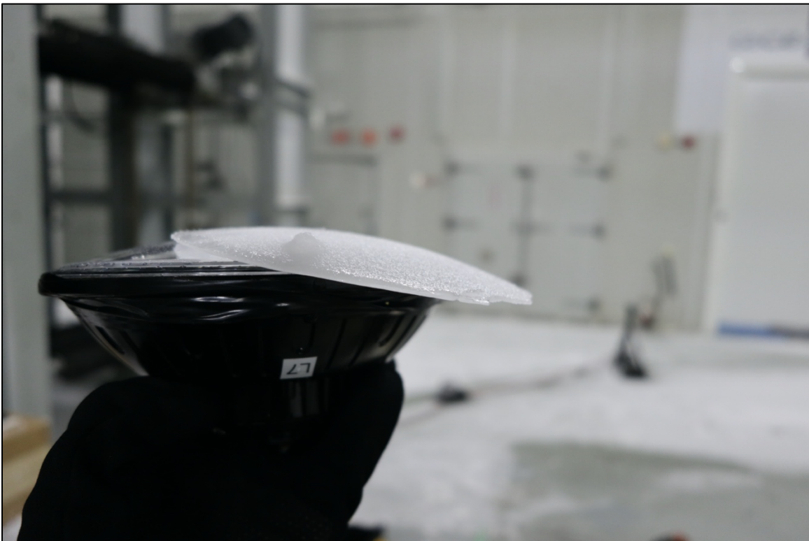
Figure 49. Documentation of ice on LED sample after Trial 2
