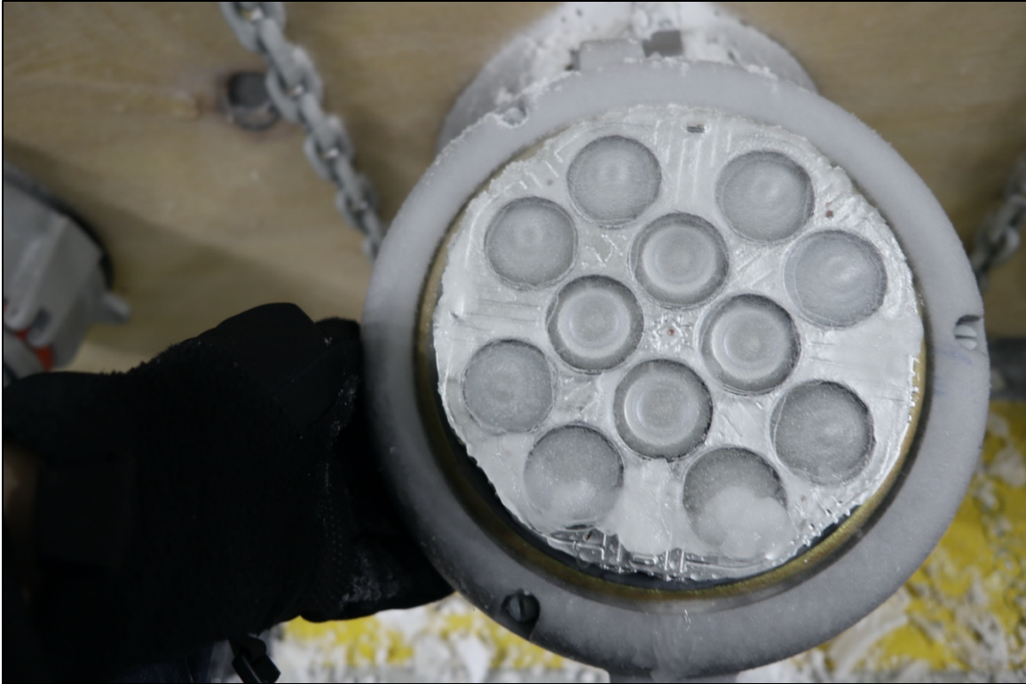
Figure 48. Documentation of ice on LED sample after Trial 2
