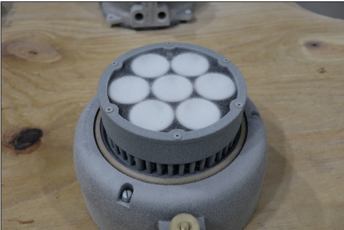
Figure 53. LED sample in the early stages of building the 1/4 inch layer of ice
