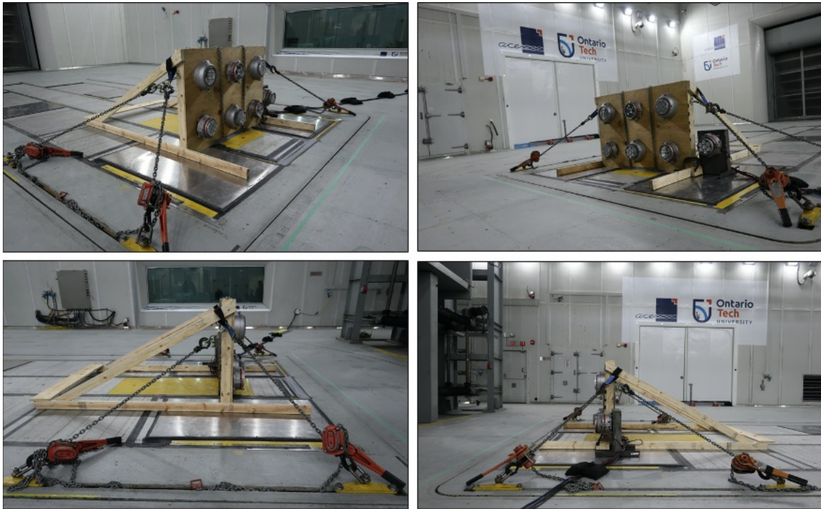
Figure 6. Test frame installed in the CWT prior to Snow Accumulation Test
