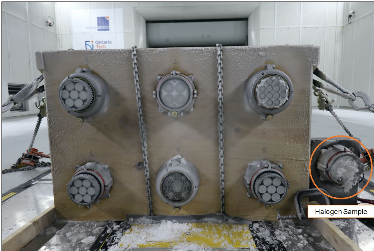
Figure 19. Accumulation of snow and ice on light fixtures after Trial 3
