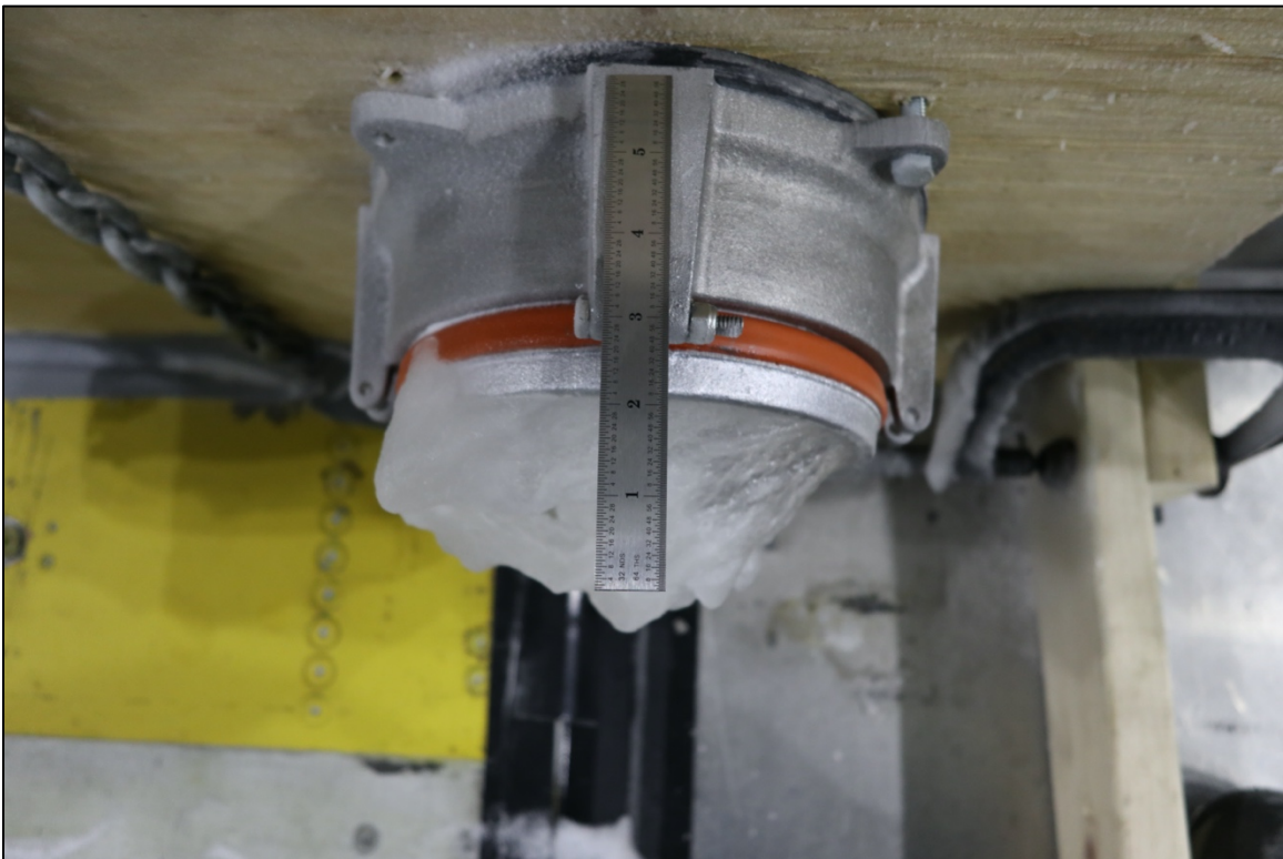
Figure 40. Measurement of ice accumulation on halogen sample after Trial 1
