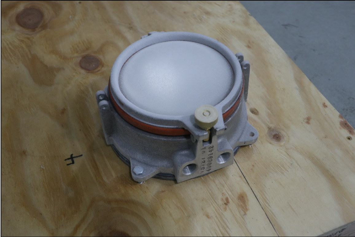
Figure 54. Halogen sample in the early stages of building the 1/4 inch layer of ice
