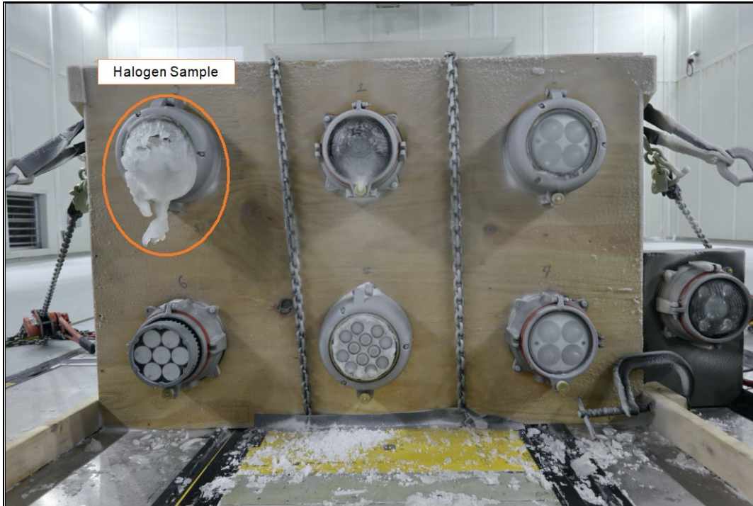
Figure 18. Accumulation of snow and ice on light fixtures after Trial 2
