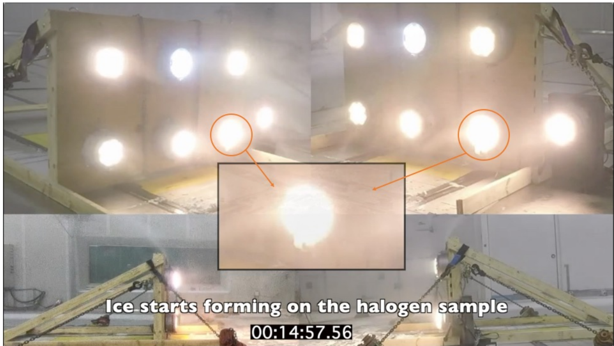
Figure 13. Photo taken during Trial 1 with detail view of halogen lamp
