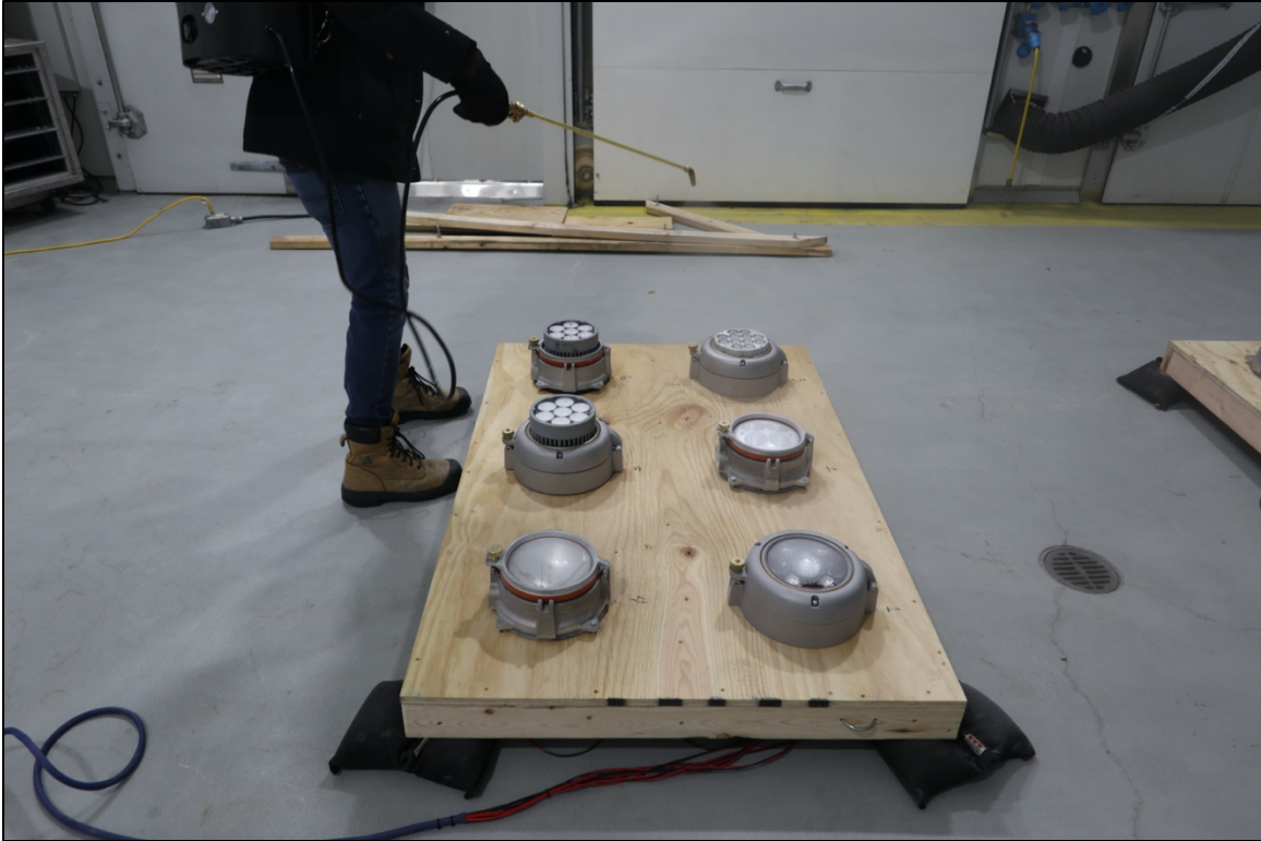
Figure 52. Early stages of the water spraying process
