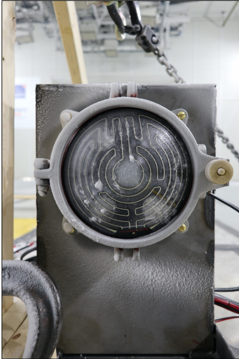
Figure 47. LED sample on metal testing frame after Trial 2
