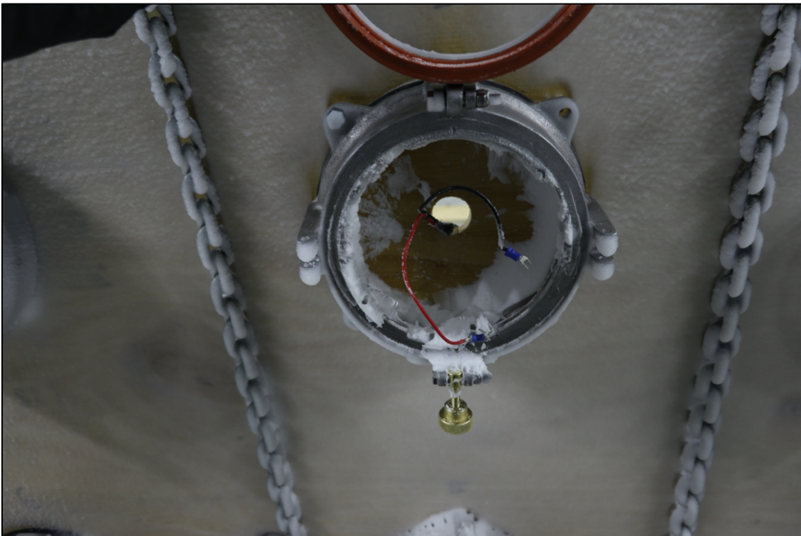
Figure 59. Documentation of snow inside housing
