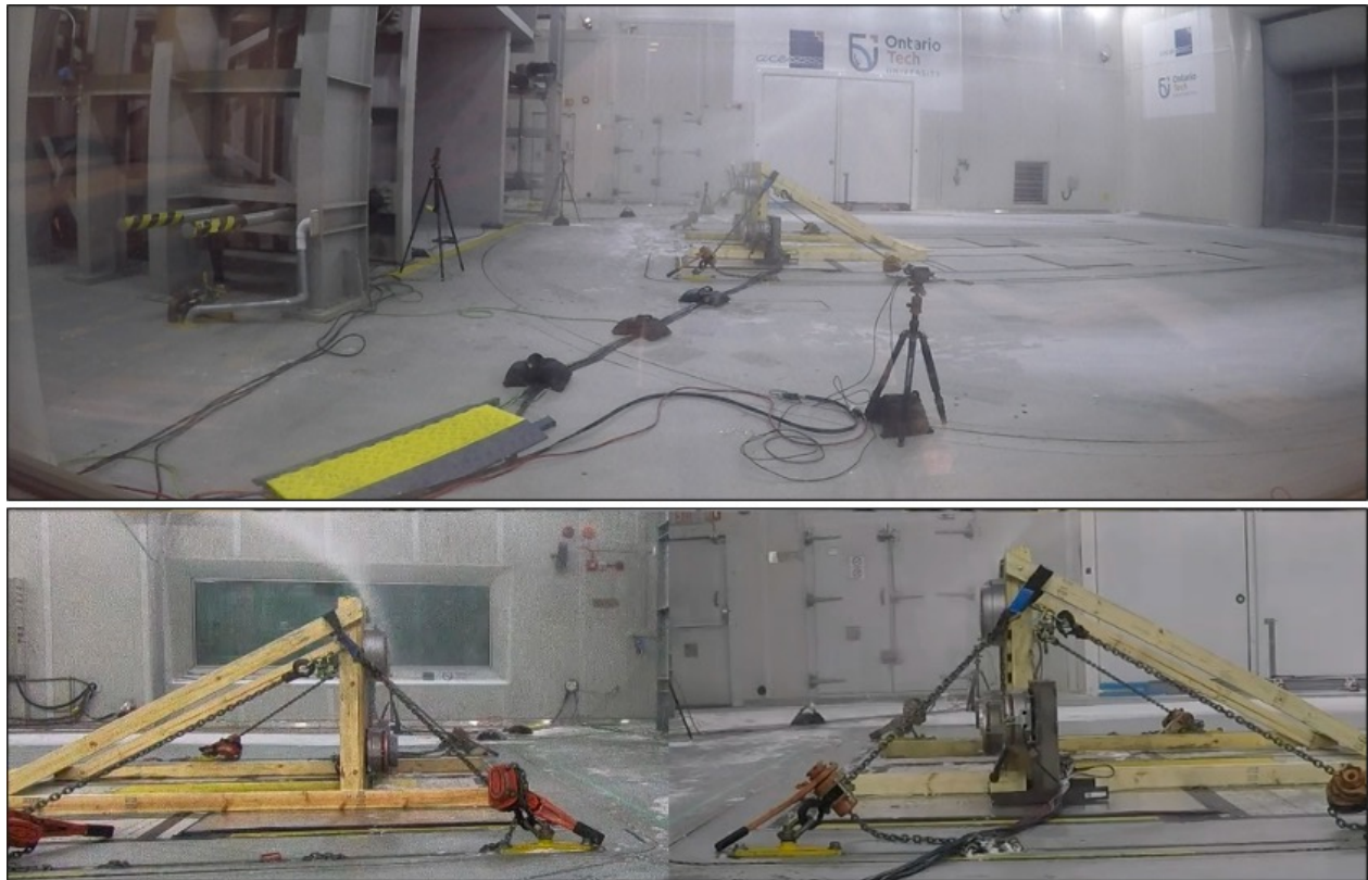
Figure 12. Test frames inside the CWT at wind speeds of 70 mph (113 km/h)
