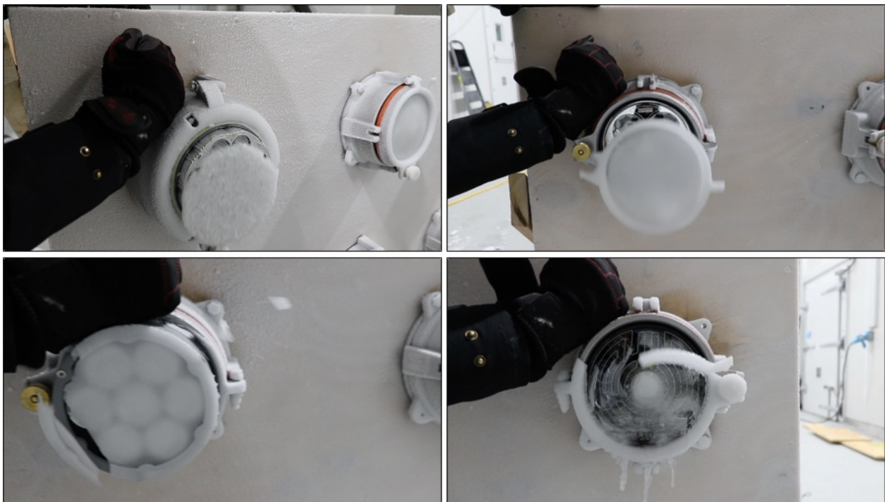
Figure 11. Layer of ice falling from lens face after moderately hitting the lamp housings
