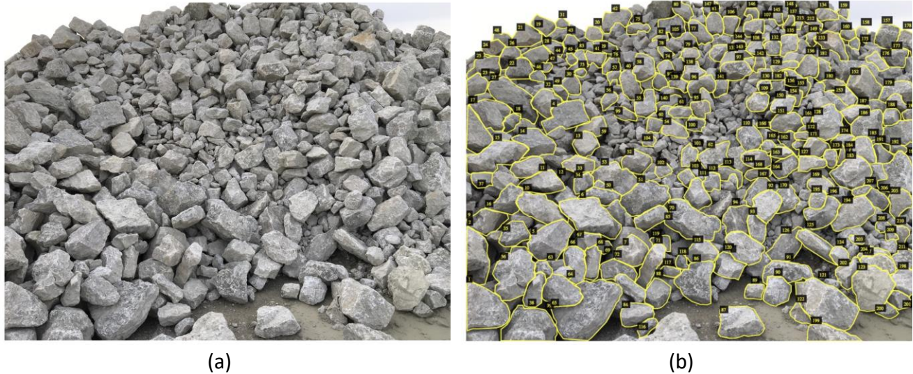
Figure 5.2. Stockpile aggregate image (a) before labeling and (b) after labeling.
