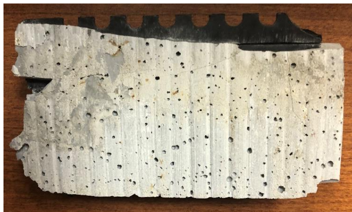
Figure 16. Dislodged R-100 with epoxy still bonded to it.
