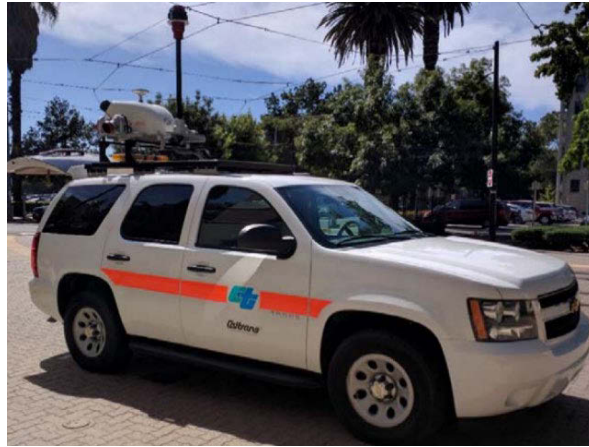
Figure 2.18 Caltrans Mobile Terrestrial Laser Scanning (MTLS) vehicle
