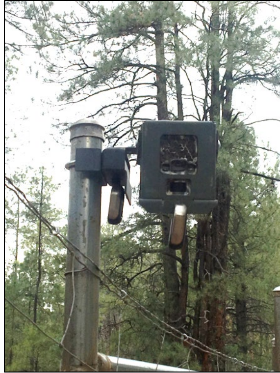
Figure 15. Camera Box Mounted to Wildlife Fencing
