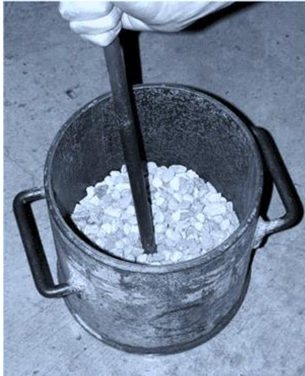
Figure 49. DRUW test in progress
