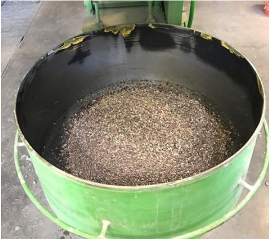
Figure 59. Coarse aggregates (#4, #8 and #10) added to the mixer
