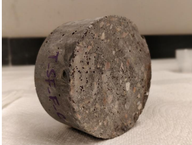
Figure 150. 50-mm thick disk sample cut from 200-mm long cylinder
