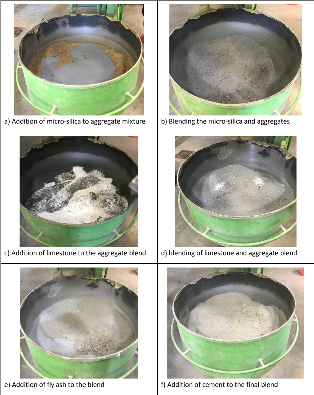
Figure 63. (a-f) Addition of powders to the aggregate mixture
