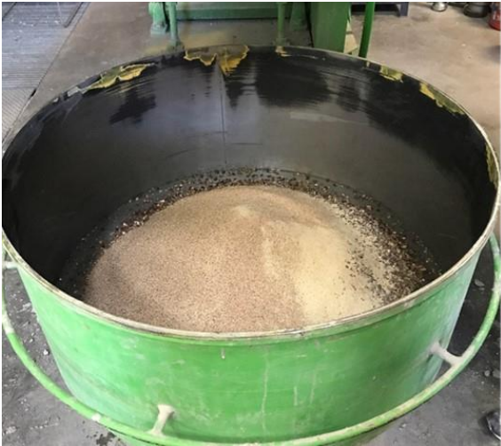
Figure 60. Fine aggregates (concrete sand and fine sand) added along with the coarse aggregates
