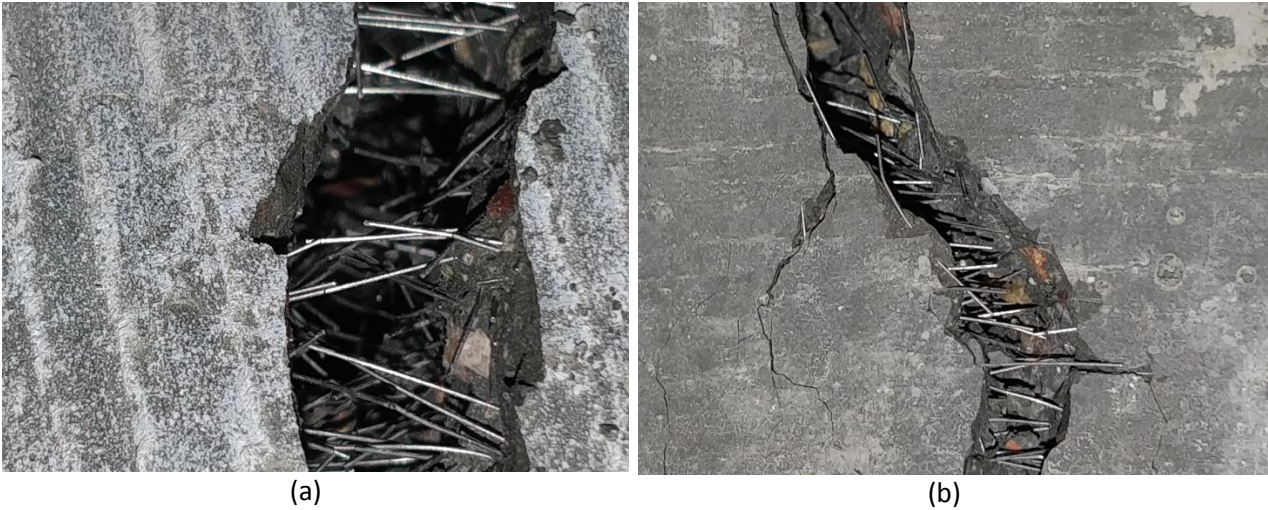
Figure 69. Bridging effect of fibers on samples with: (a) 1% fiber content; (b) 3% fiber content
