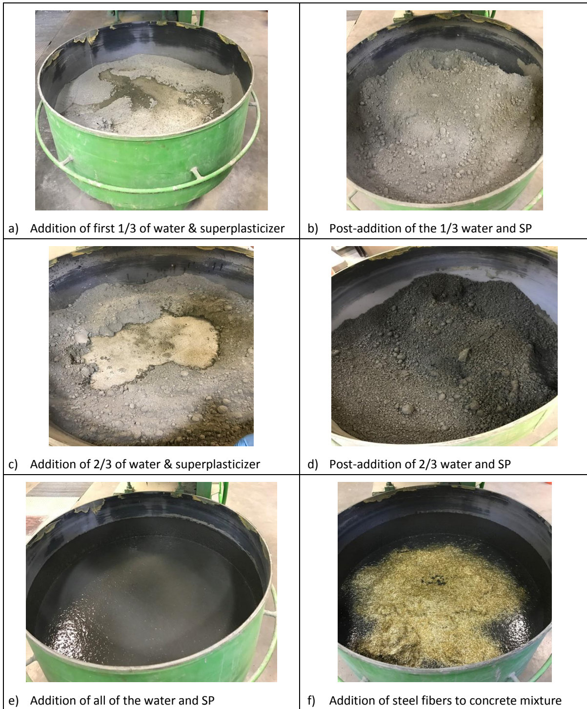
Figure 64. (a-f) Addition of water, superplasticizer (SP) and fibers to the mixture
