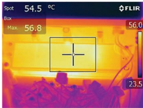
Figure 5.2 Driver thermal profile.
