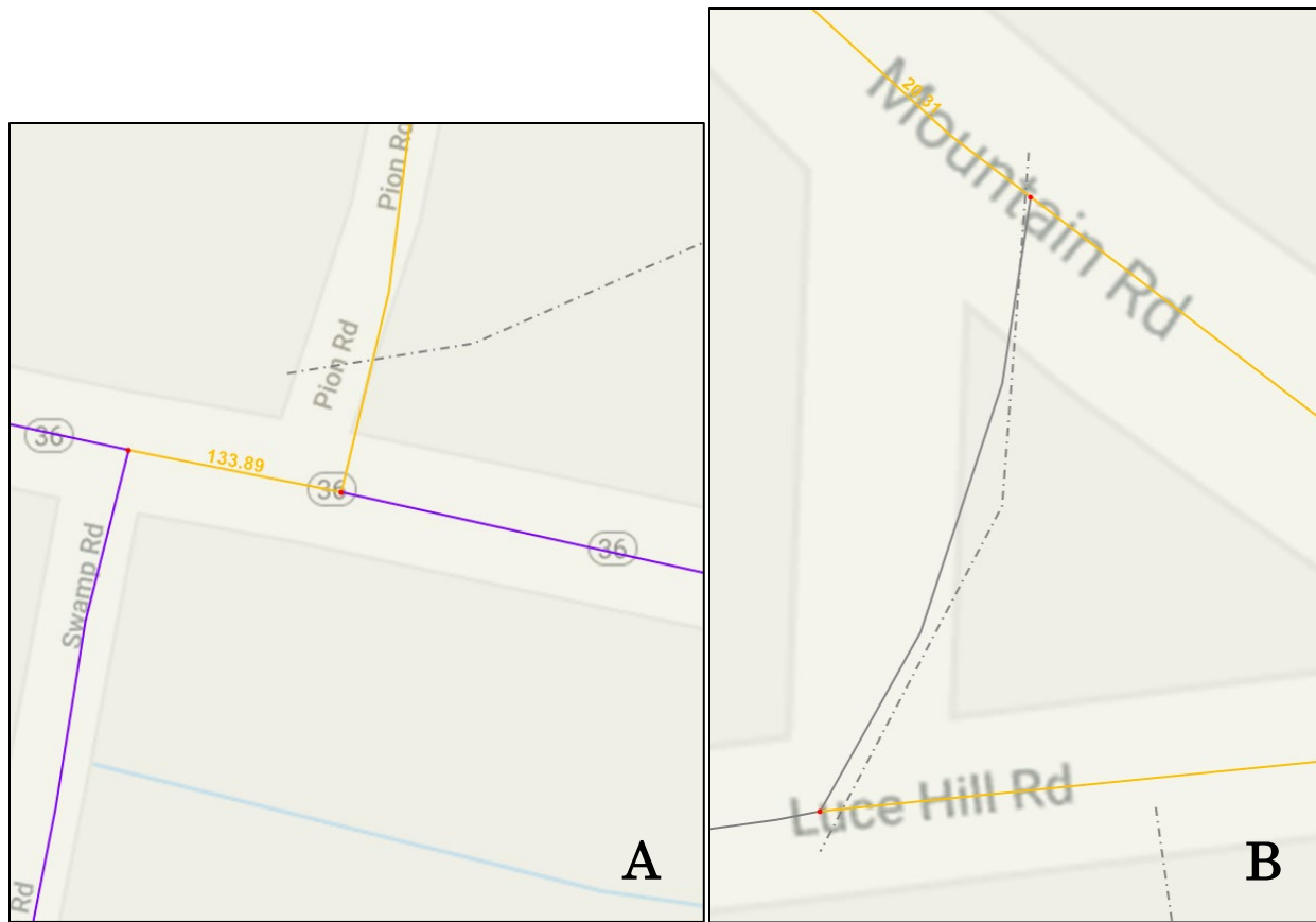
Figure 1 A - Driveway (Dashed Line) Assigned to Two Segments (in Yellow) and B - Driveway Already Represented in the Roadway Layer
