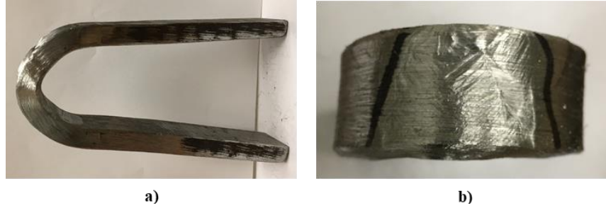
Figure 15. a) Side view and b) top view of the side bend samples with the weld placed in the middle
