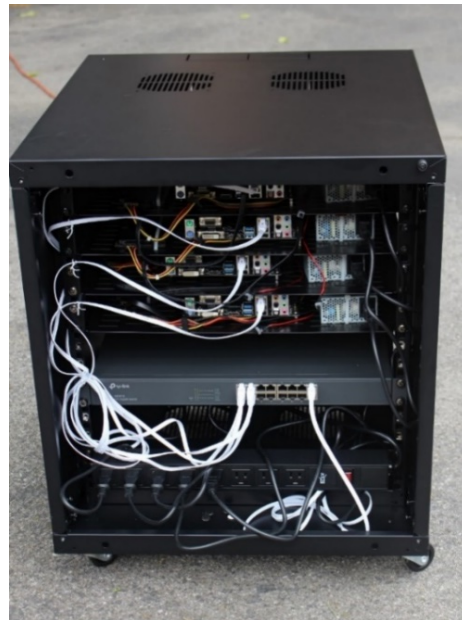
Fig. 2.2. Modular data collection system in which the SBCs are placed at the top of the rack, the network switch is in the middle of the rack, and power distribution and batteries are at the bottom of the rack
