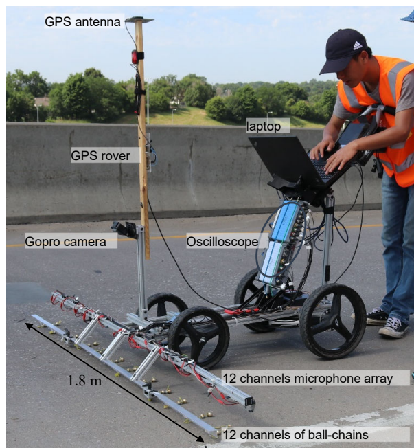
Fig. 3.4. 12-channel acoustic scanning cart
