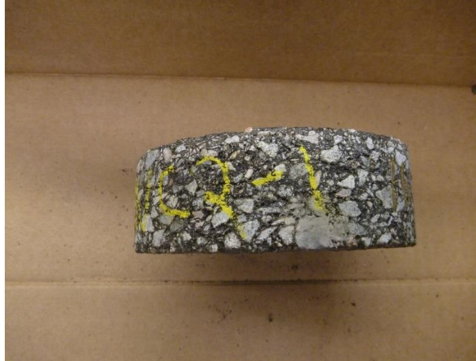
Figure 17. Core Showing Microsurfacing Above Existing Asphalt Top Surface
