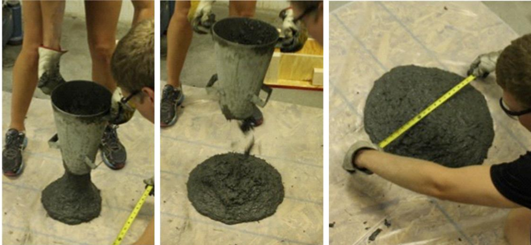
Figure 15. Inverted Cone Slump Testing
