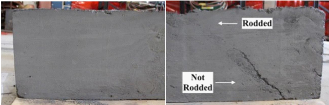
Figure 63. Shear Key Flow Test Lower End (Left) and Upper End (Right)
