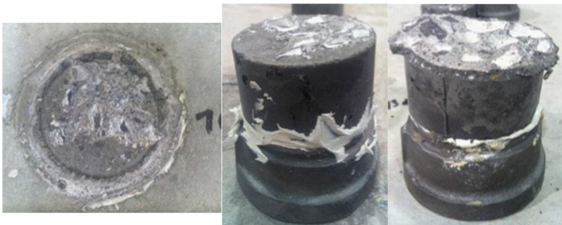
Figure 59. Typical VHPC 7-Days and Older Failure
