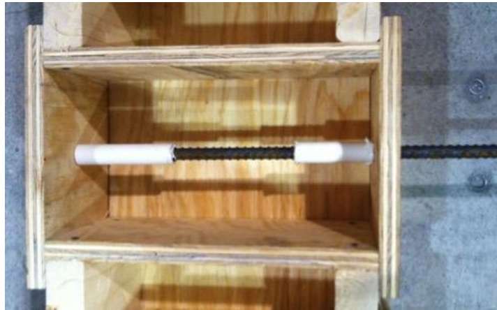
Figure 9. Bonded versus Debonded Reinforcing Steel for Pull Out Specimen
