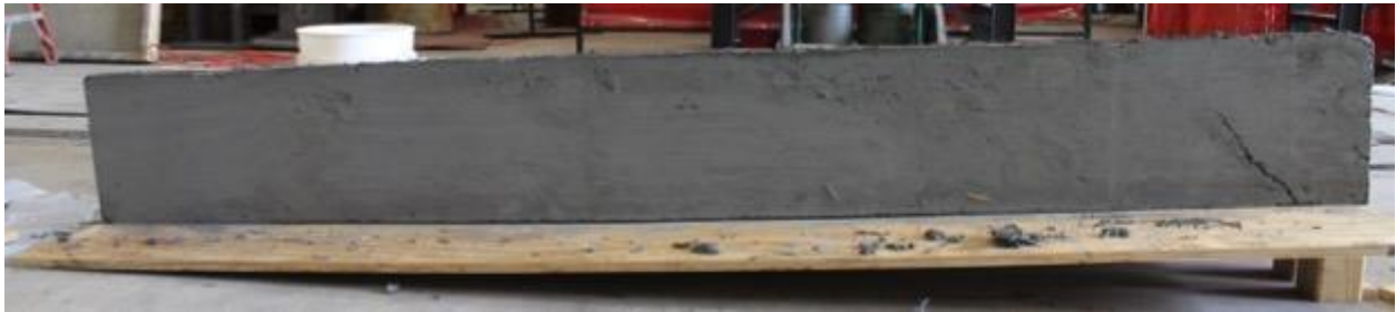
Figure 62. Shear Key Flow Test Overall After Removing the Formwork
