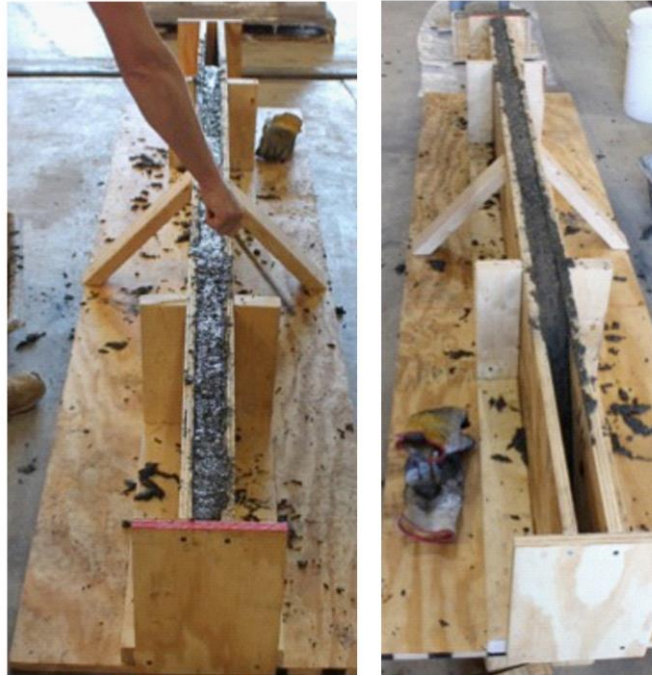
Figure 17. Shear Key Flow Test
