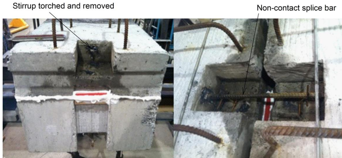
Figure 20. Non-Contact Voids Slab Connection
