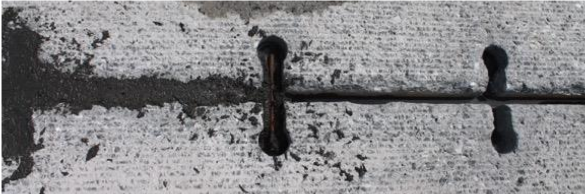
Figure 100. Reinforcing Steel in Dog Bone
