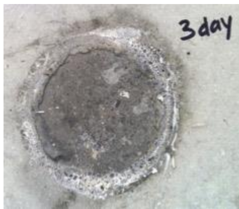
Figure 58. Typical VHPC 2-Day to 5-Day Failure
