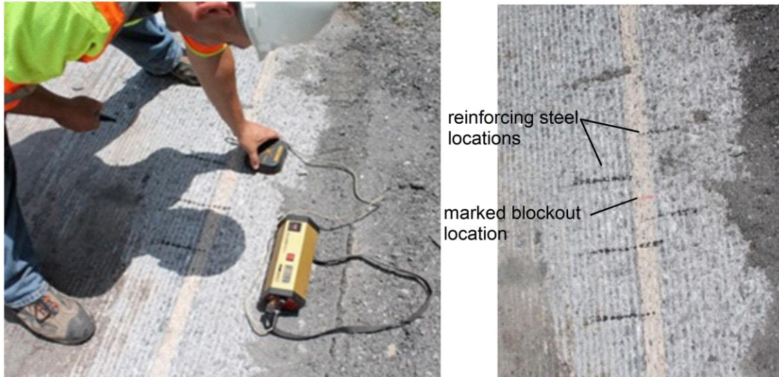
Figure 92. Locating Steel with Pachometer and Marking
