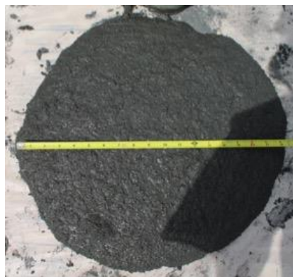
Figure 98. Slump Test, VHPG Target Spread of 18 in
