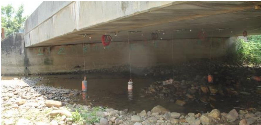
Figure 23. Concrete Cylinders Weighing Down Wires Used for Pre-deflection
