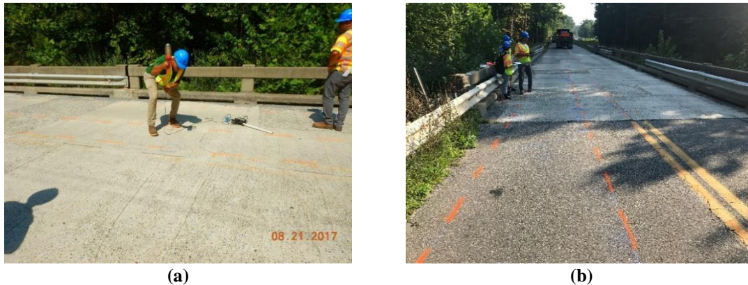
Figure 6 – Representation of Excitation Methods Used During Vibration Testing: (a) impact hammer excitation; (b) ambient excitation
