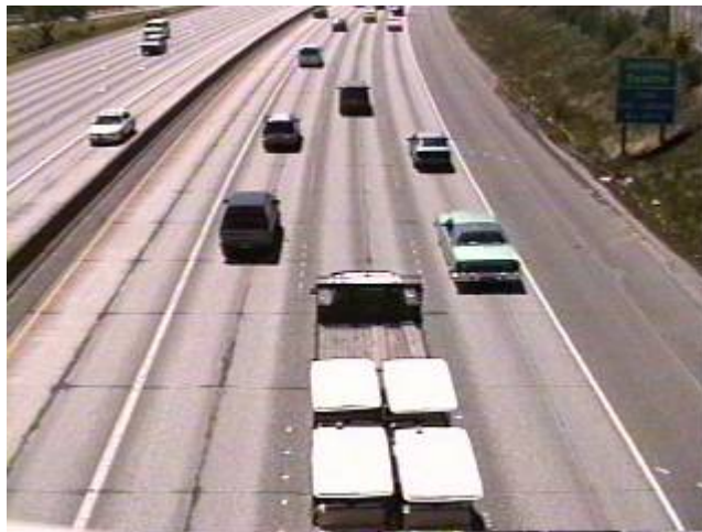
Figure 7-7: A Misclassified Truck with the Color of the Bed Similar to the Background Color
