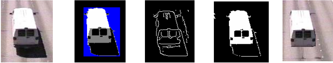
Figure 6-9: A Step by Step Illustration of the Shadow Removal Process (from left to right): (a) Original Image; (b) Bounding Box Area (Shown in Blue); (c) Detected Edges; (d) Shadow Identification; and (e) Shadow Removal.
