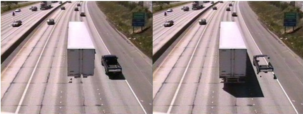
Figure 5-3: Otsu Method for Shadow Removal on a Bright Vehicle and a Dark Vehicle
