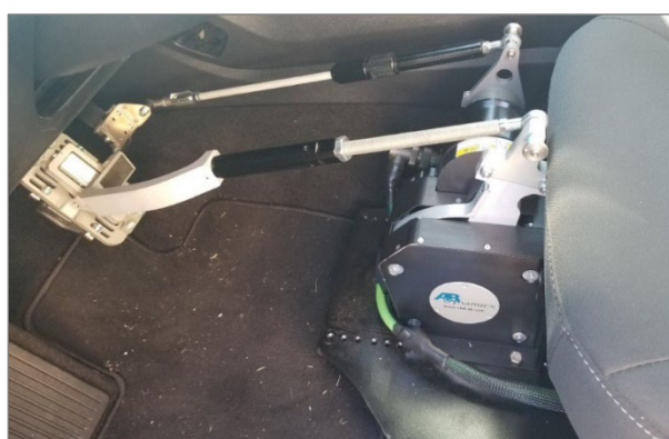
Figure 2-4. Example robotic brake and accelerator controller installation used in SV and LV.
