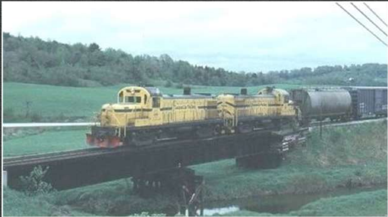
The LVRC chopped the noses on some of their RS3s. 1981 Photo by Paul Charland
