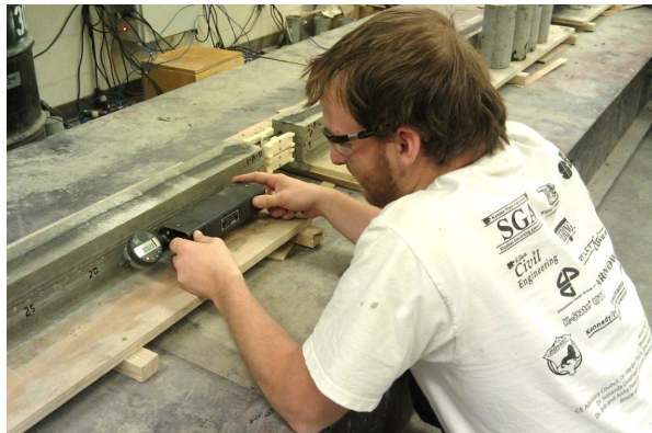
Figure 4: Measurement of concrete surface displacements using a Whittemore gage
