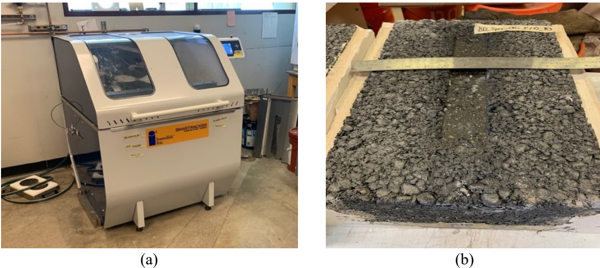
Figure 5.17: Hamburg wheel tracking test (a) Test system used for conducting experiments (b) Tested block sample.
