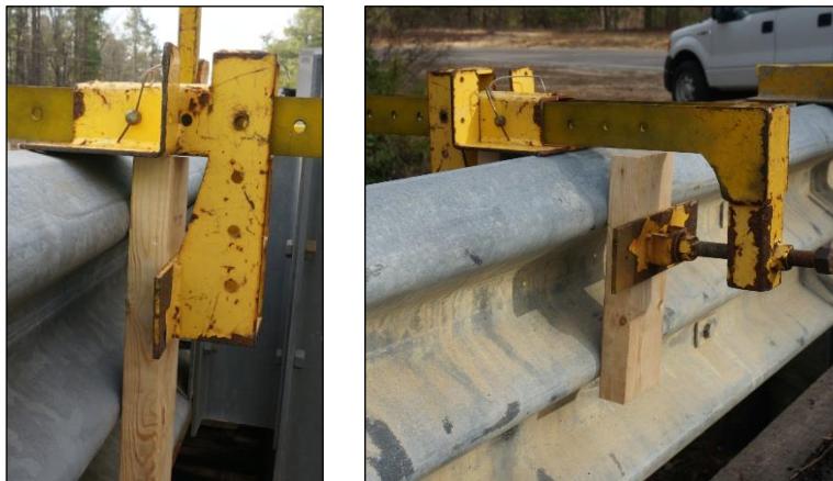
Figure 5. Sample FPSD installation with lumber blocks
