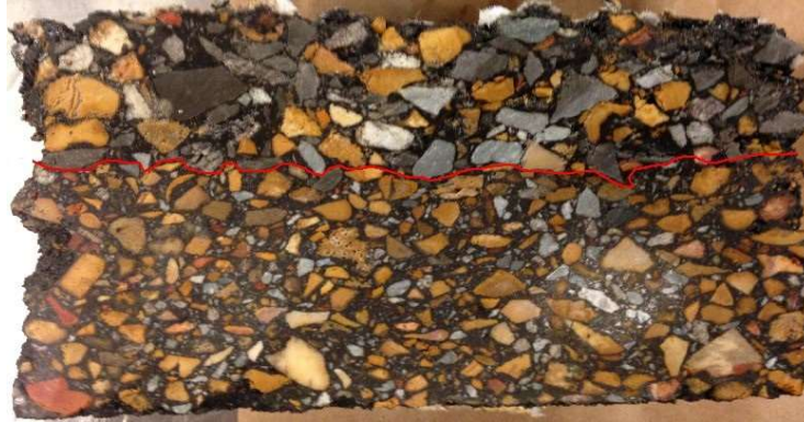
Figure 4- 25 Section combined by OGFC and TLD
