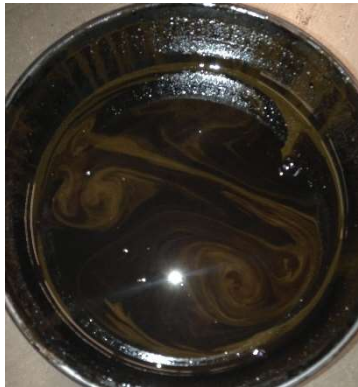
Figure 3- 4 Ultrafuse tack coat
