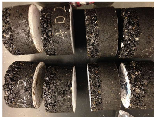
Figure 3- 12 Specimens for shear test and fatigue test
