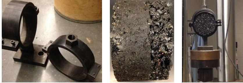
Figure 3- 7 Shear test setup and sample
