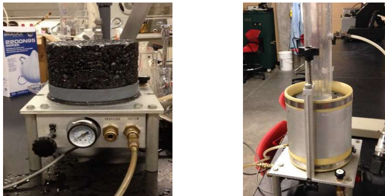
Figure 3- 6 Permeability test setup and sample
