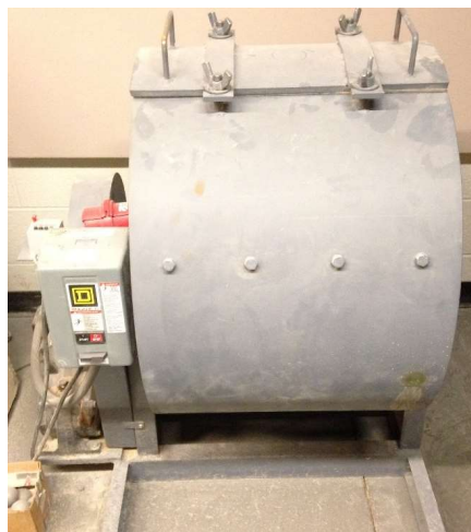
Figure 3- 5 Los Angeles Abrasion machine
