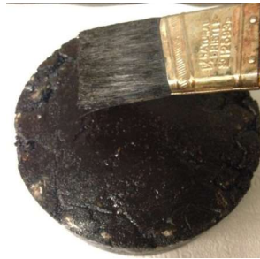
Figure 3- 11 Tack coat was applied on the upper surface of underlying layer
