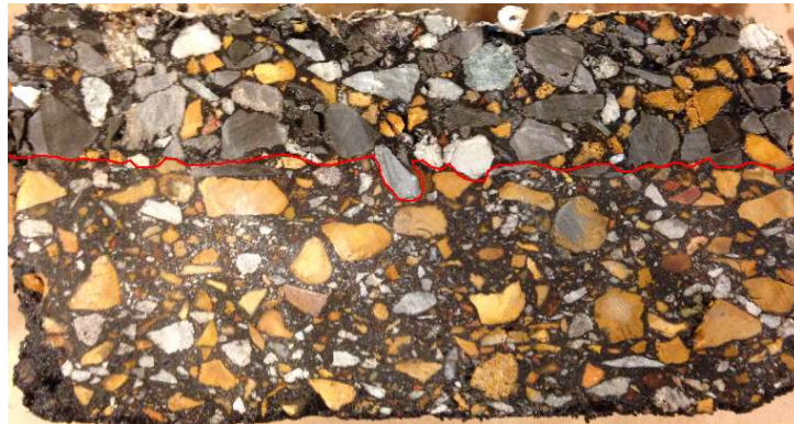
Figure 4- 26 Section combined by OGFC and D
