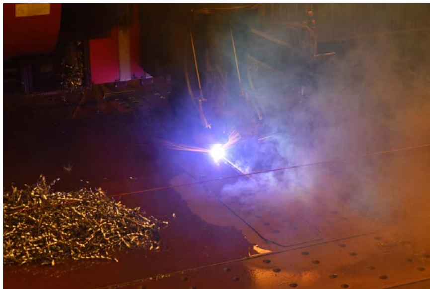
Figure 4: CNC machine plasma cutting a splice plate
