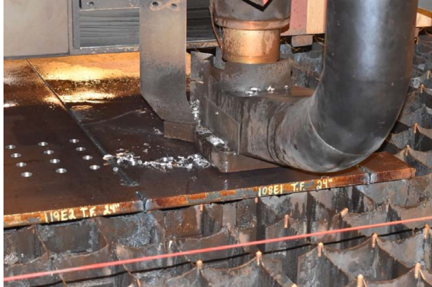
Figure 3: CNC machine drilling a splice plate
