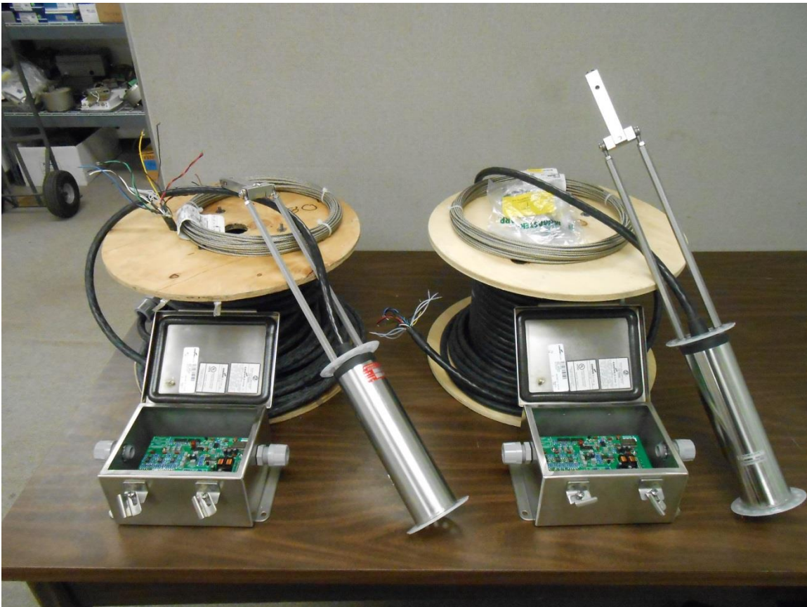
Figure 13. Two borehole sensors packages before installation.
